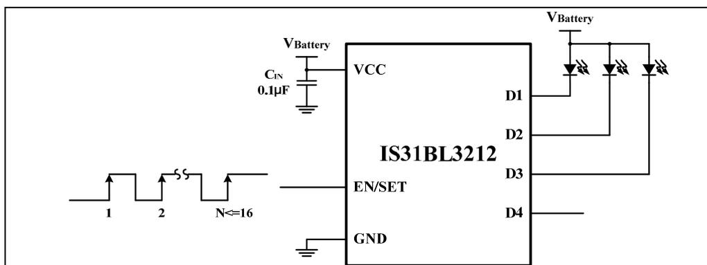
Figure 2 Application Circuit for Less Than 4 LEDs
