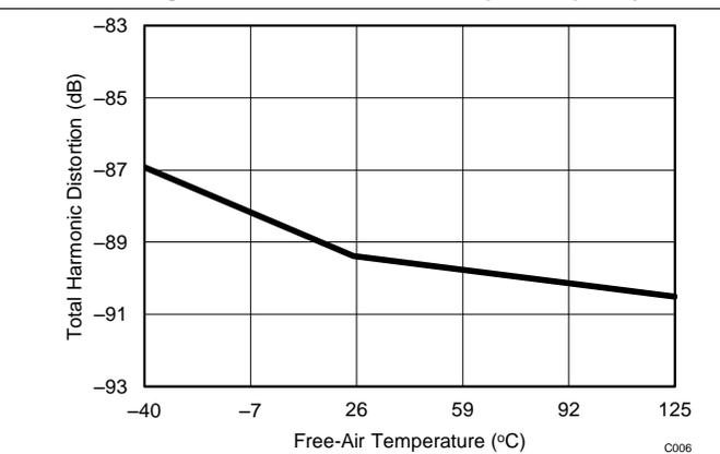
Figure 7. THD vs Free-Air Temperature
