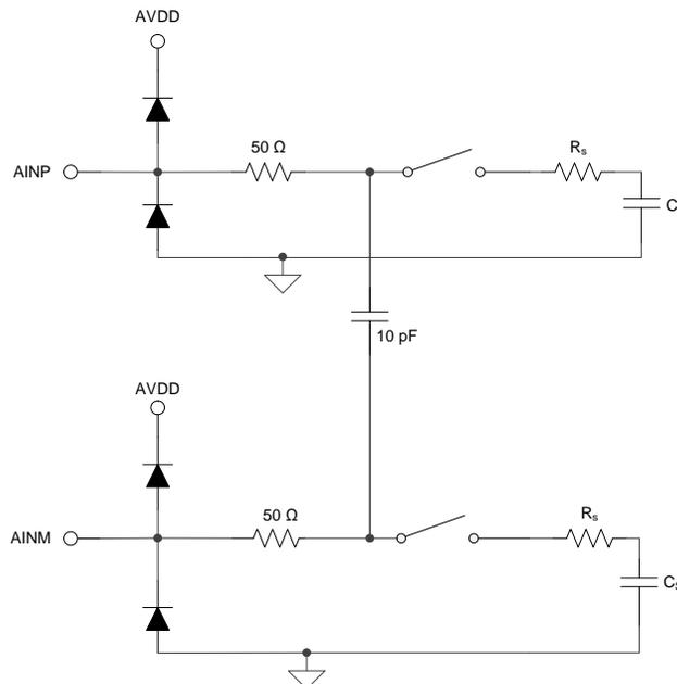
Figure 33. Equivalent Input Circuit for the Sampling Stage
