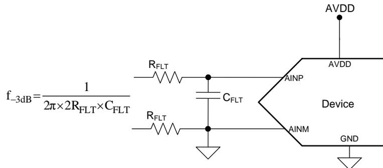
**Figure 40. Antialiasing Filter**
