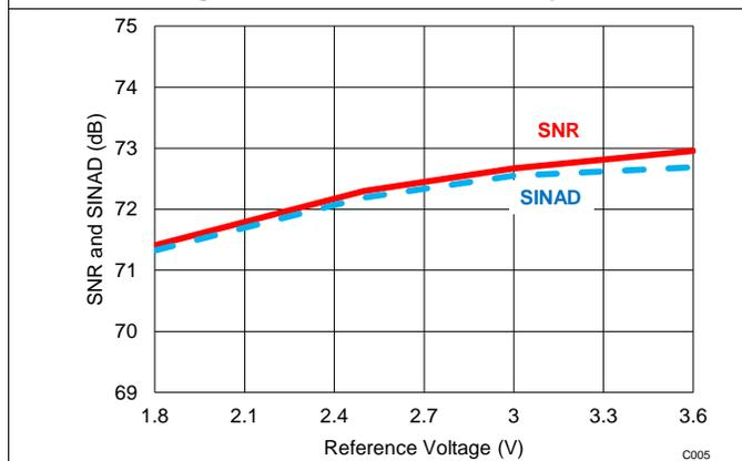
Figure 6. SNR and SINAD vs Reference Voltage (AVDD)
