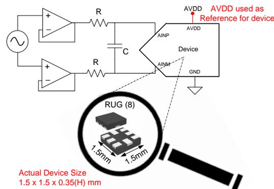
NOTE: The device is smaller than a 0805 (2012 metric) SMD component.
