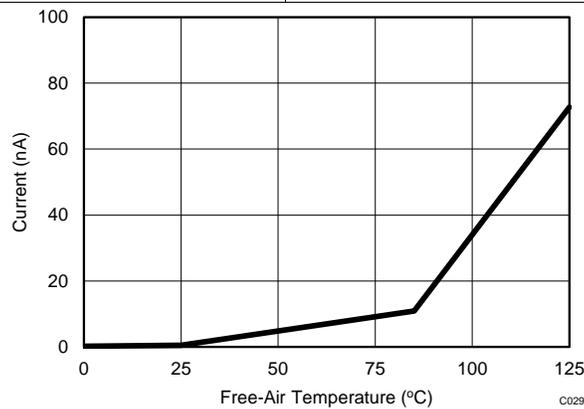
Figure 30. AVDD Static Current vs Free-Air Temperature
