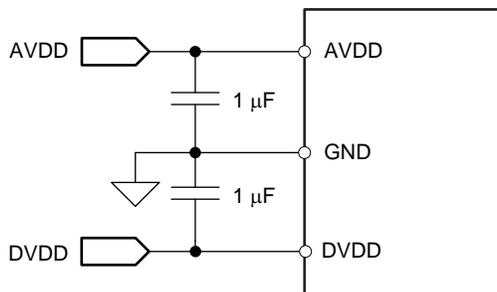
**Figure 45. Power-Supply Decoupling**
