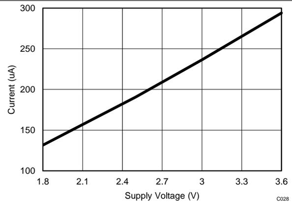
Figure 29. AVDD Supply Current vs AVDD Voltage
