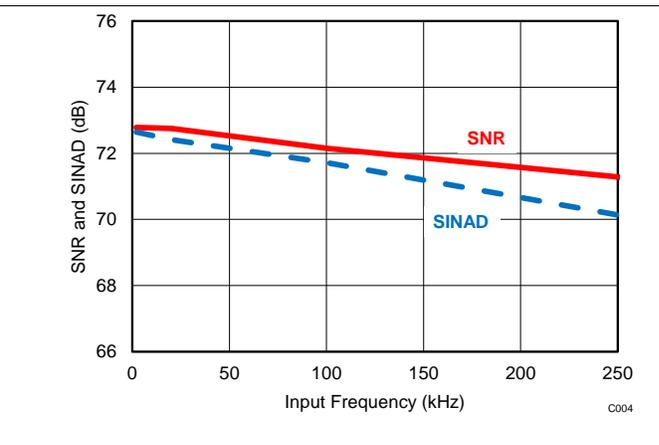
Figure 5. SNR and SINAD vs Input Frequency
