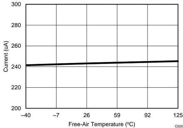
Figure 26. AVDD Supply Current vs Free-Air Temperature
