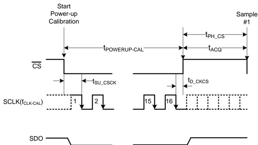
Figure 37. Offset Calibration on Power-Up Timing Diagram
