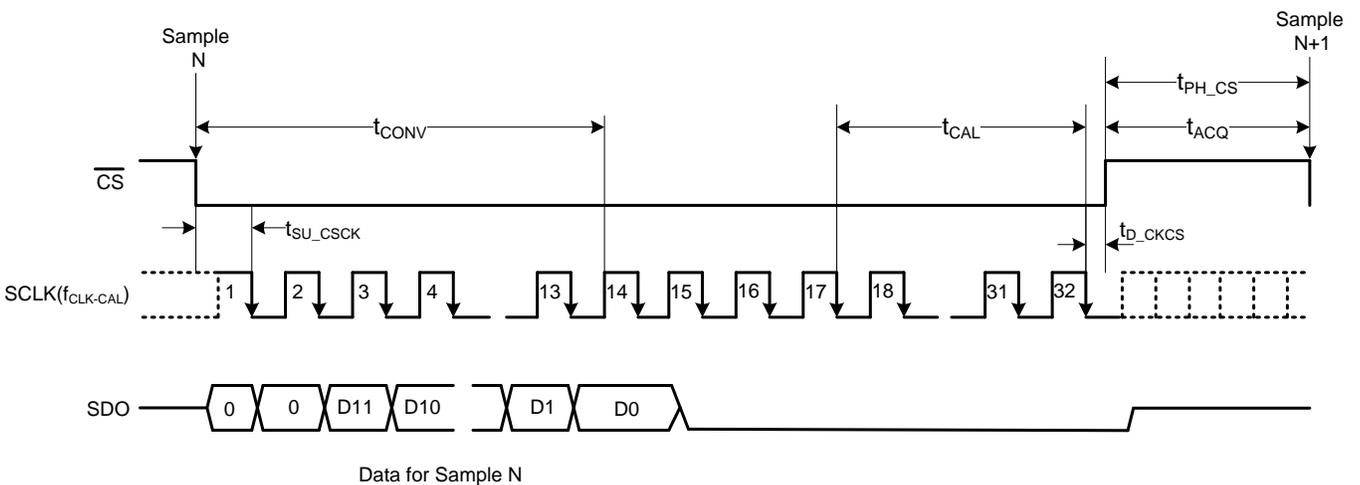
**Figure 38. Offset Calibration During Normal Operation Timing Diagram**
