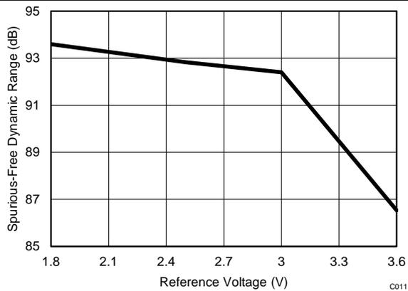
**Figure 12. SFDR vs Reference Voltage (AVDD)**
