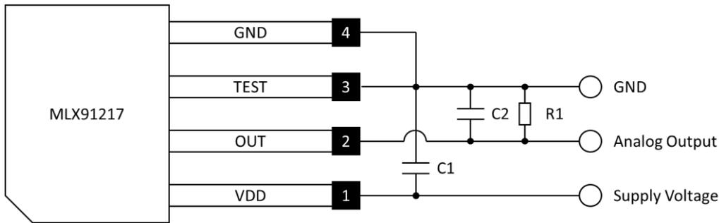
Figure 4: Application Diagram with external Pull-Down resistance
