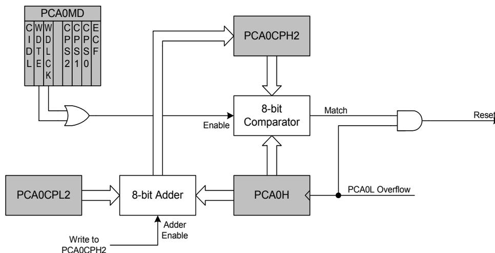
Note that the 8-bit offset held in PCA0CPH2 is compared to the upper byte of the 16-bit PCA counter. This offset value is the number of PCA0L overflows before a reset. Up to 256 PCA clocks may pass before the first PCA0L overflow occurs, depending on the value of the PCA0L when the update is performed. The total offset is then given (in PCA clocks) by Equation 19.4, where PCA0L is the value of the PCA0L register at the time of the update.
