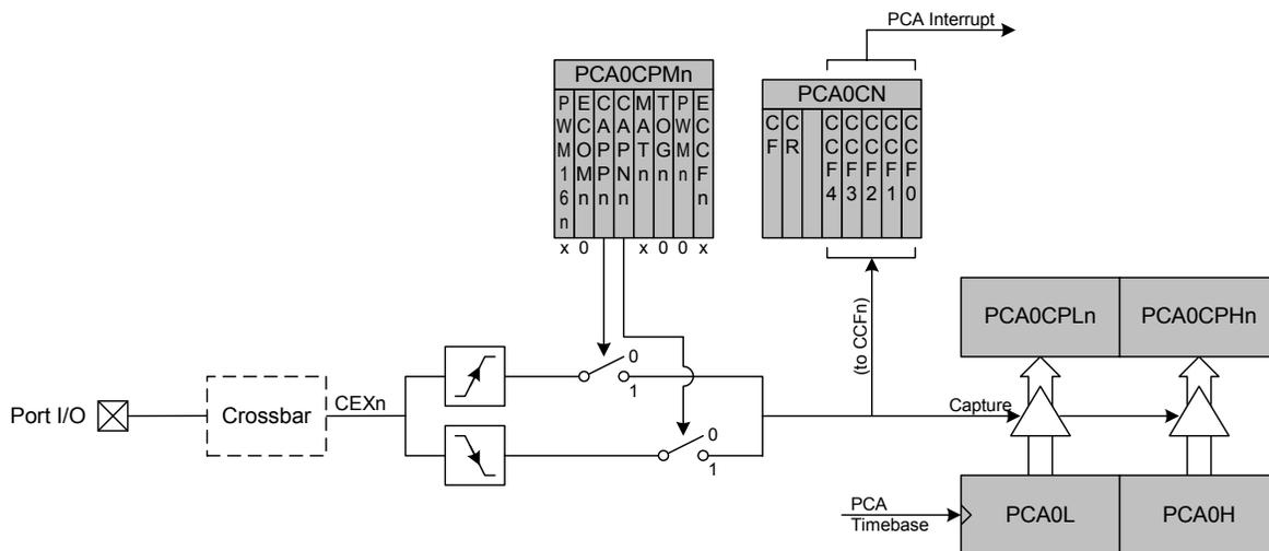
Note: The CEX<sub>n</sub> input signal must remain high or low for at least 2 system clock cycles to be recognized by the hardware.
