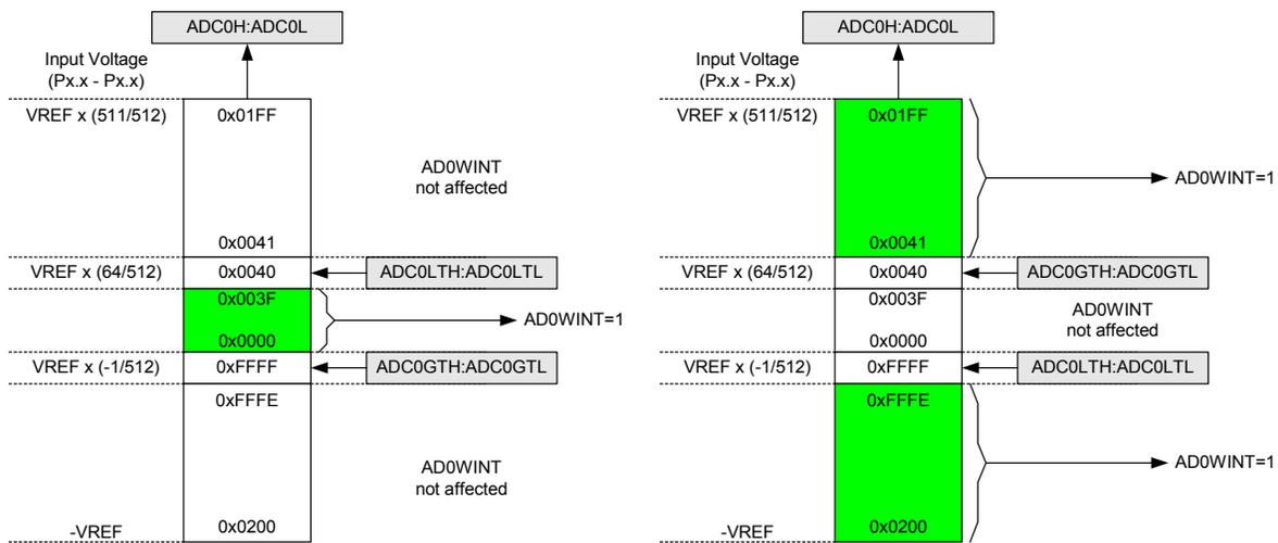
**Figure 5.18. ADC Window Compare Example: Left-Justified Differential Data**
