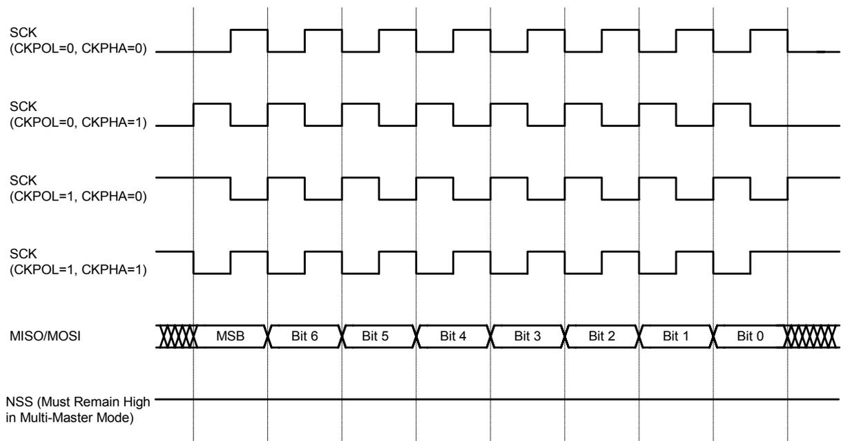
**Figure 17.6. Slave Mode Data/Clock Timing (CKPHA = 0)**
