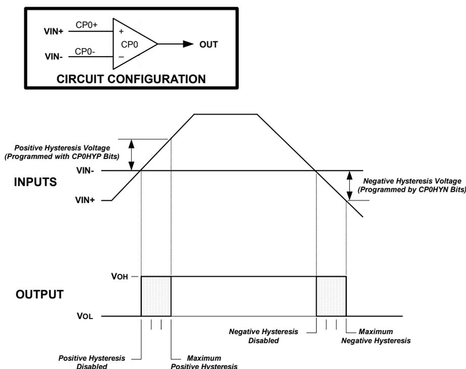
The Comparator hysteresis is software-programmable via its Comparator Control register CPT0CN. The user can program both the amount of hysteresis voltage (referred to the input voltage) and the positive and negative-going symmetry of this hysteresis around the threshold voltage.
