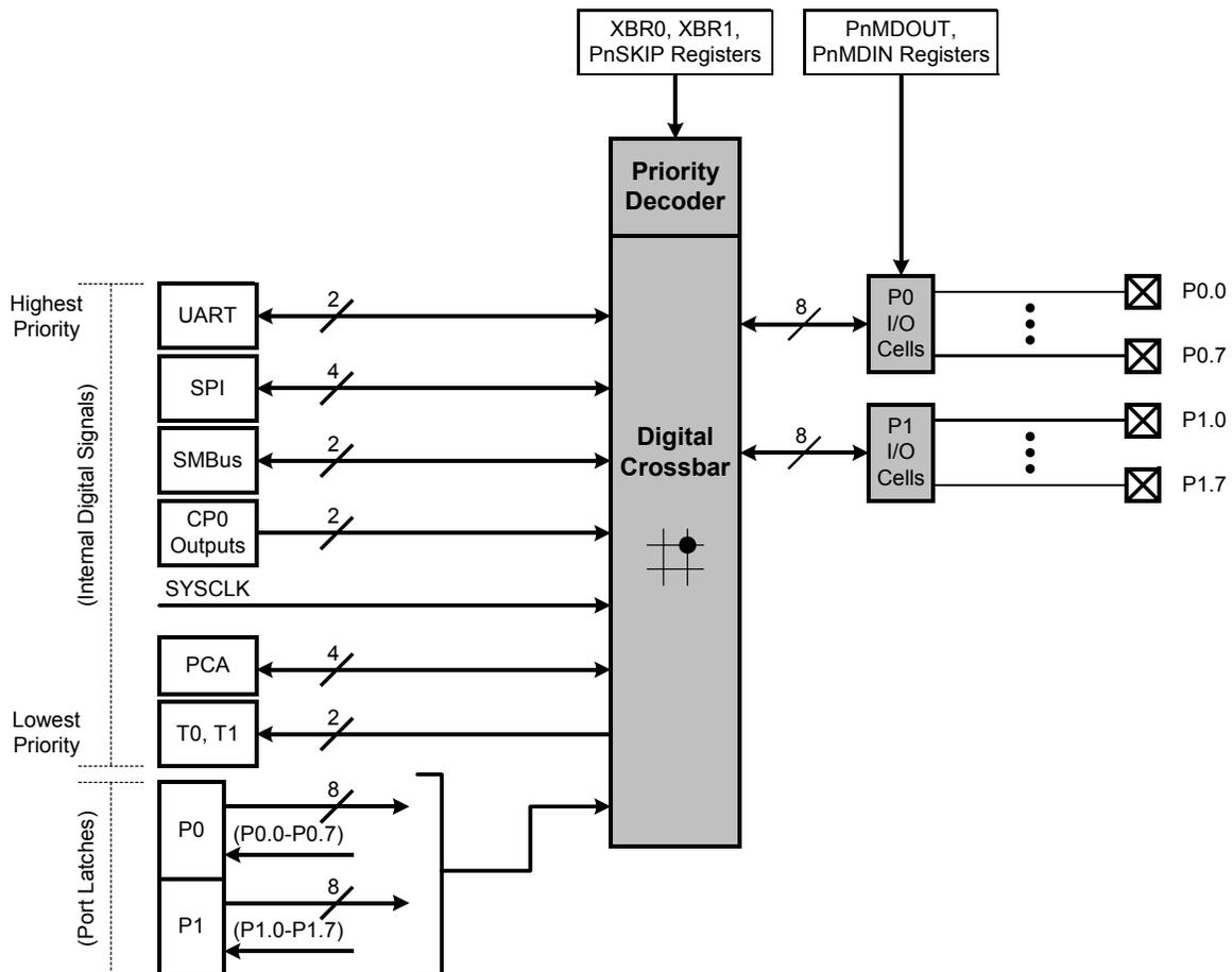
**Figure 14.2. Port I/O Cell Block Diagram**
