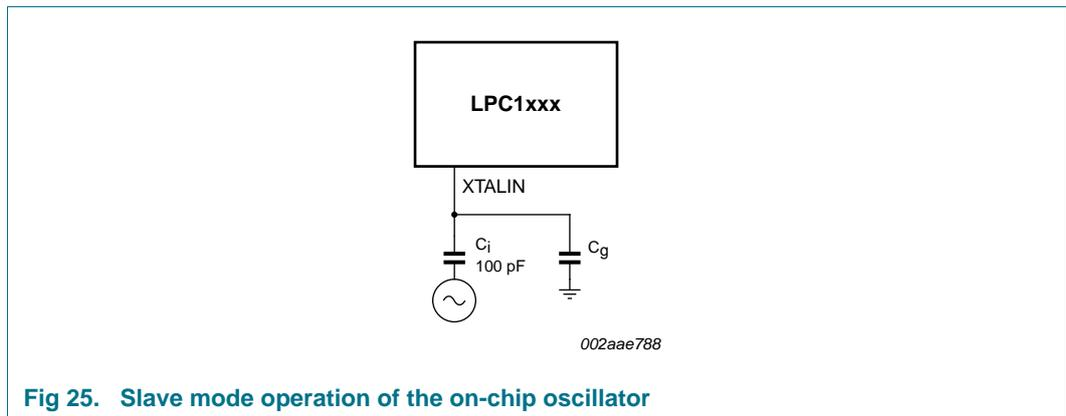
**Fig 25. Slave mode operation of the on-chip oscillator**
