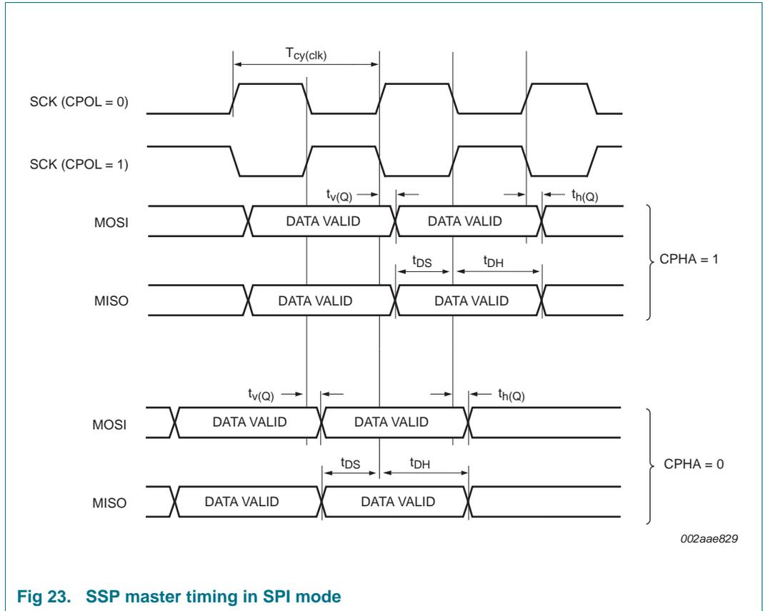
Fig 23. SSP master timing in SPI mode
