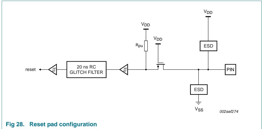
Fig 28. Reset pad configuration
