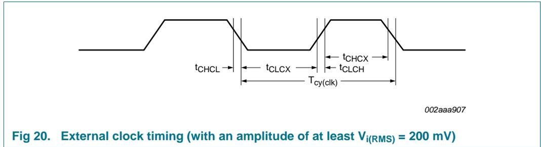
Fig 20. External clock timing (with an amplitude of at least  $V_{i(RMS)} = 200\text{ mV}$ )
