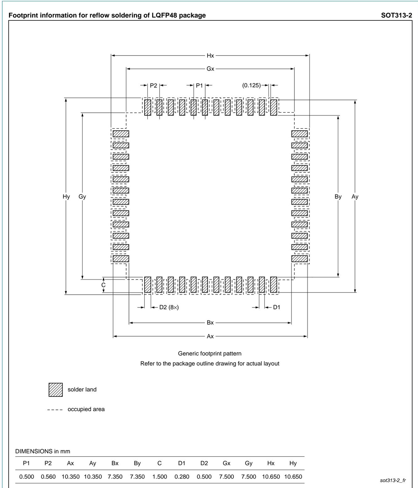
**Fig 34. Reflow soldering for the LQFP48 package**
