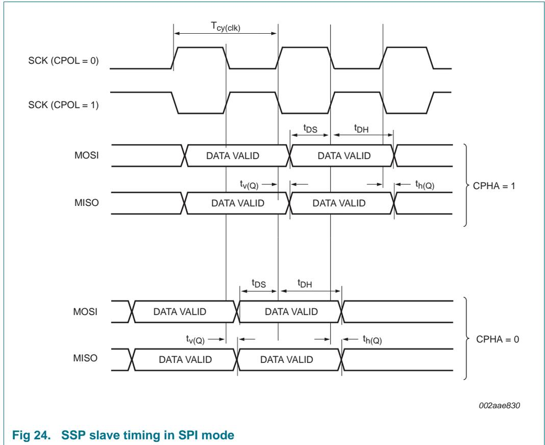
Fig 24. SSP slave timing in SPI mode
