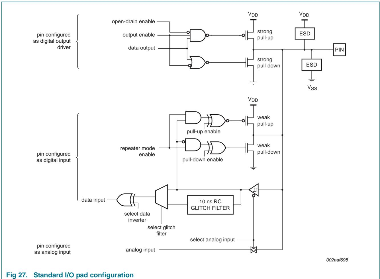
Fig 27. Standard I/O pad configuration
