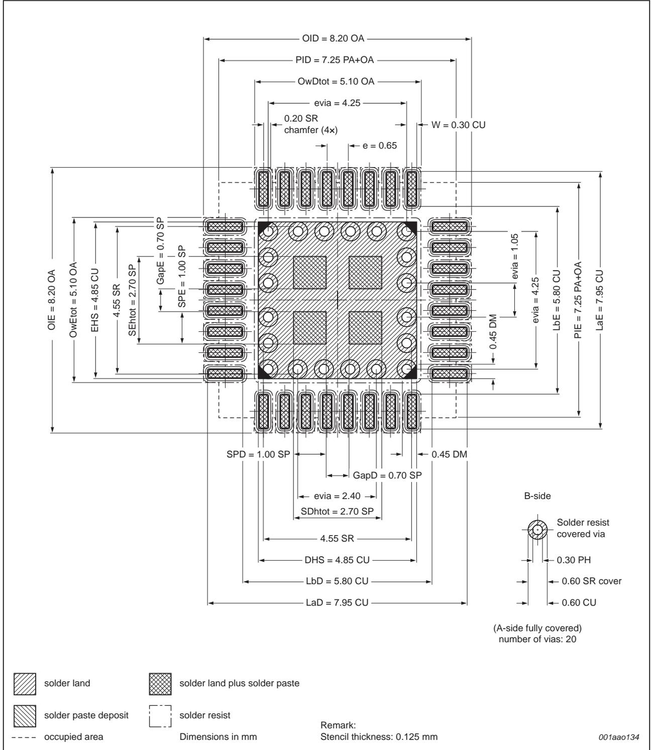
Fig 33. Reflow soldering for the HVQFN33 (7x7) package
