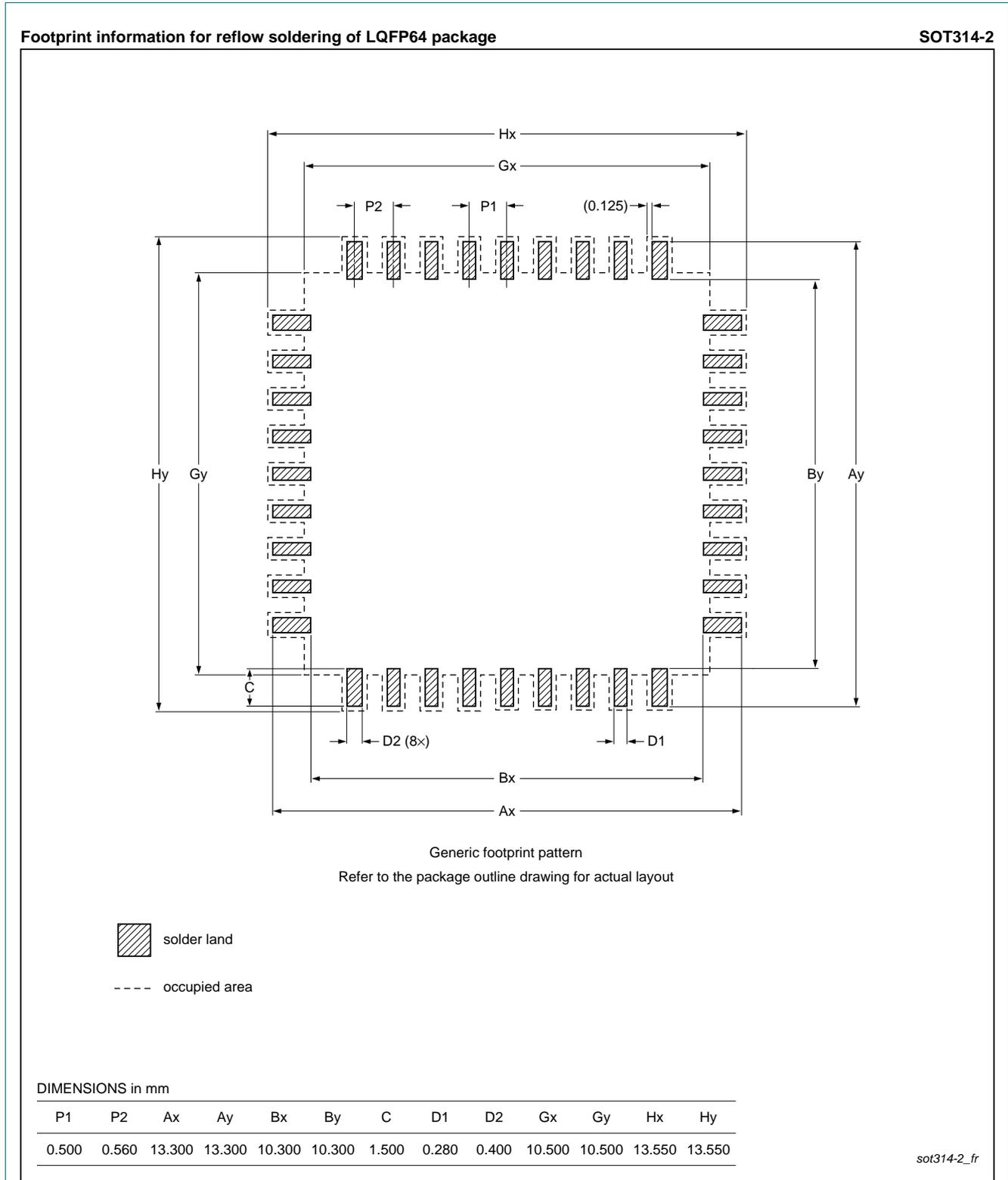
**Fig 35. Reflow soldering for the LQFP64 package**
