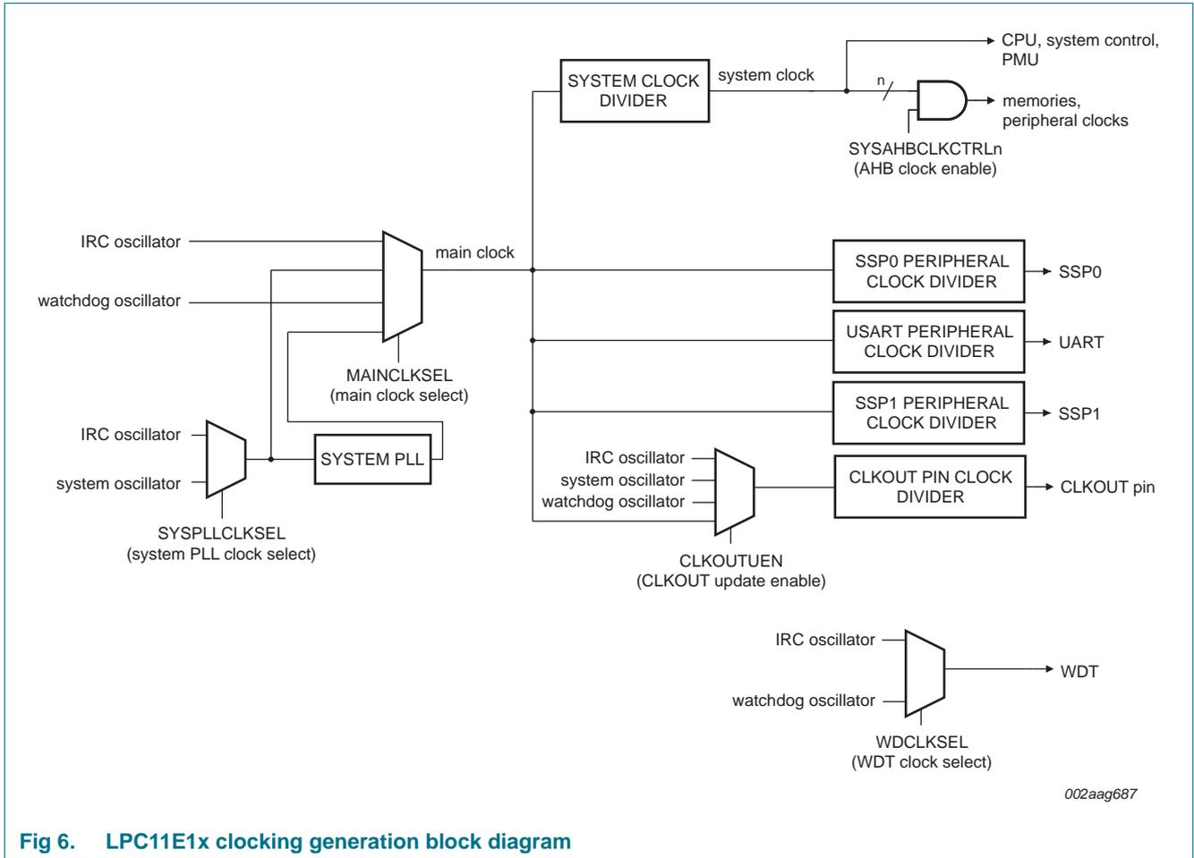
Fig 6. LPC11E1x clocking generation block diagram
