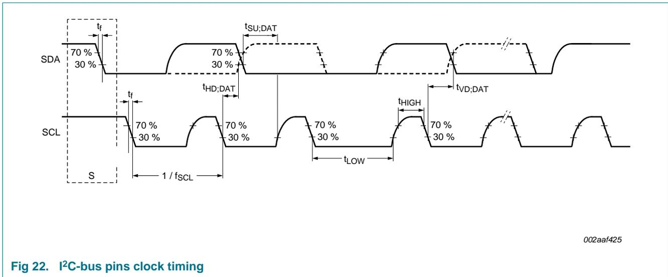
Fig 22. I<sup>2</sup>C-bus pins clock timing
