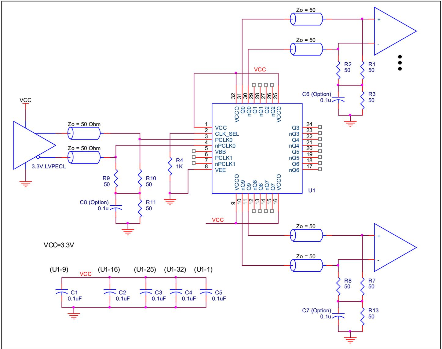
Figure 8. 853S111B Example LVPECL Clock Output Buffer Schematic
