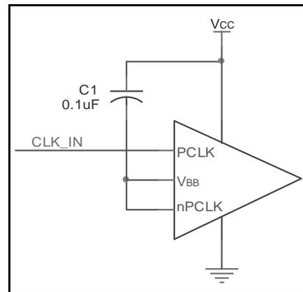
Figure 2. Single-Ended LVPECL Signal Driving Differential Input
