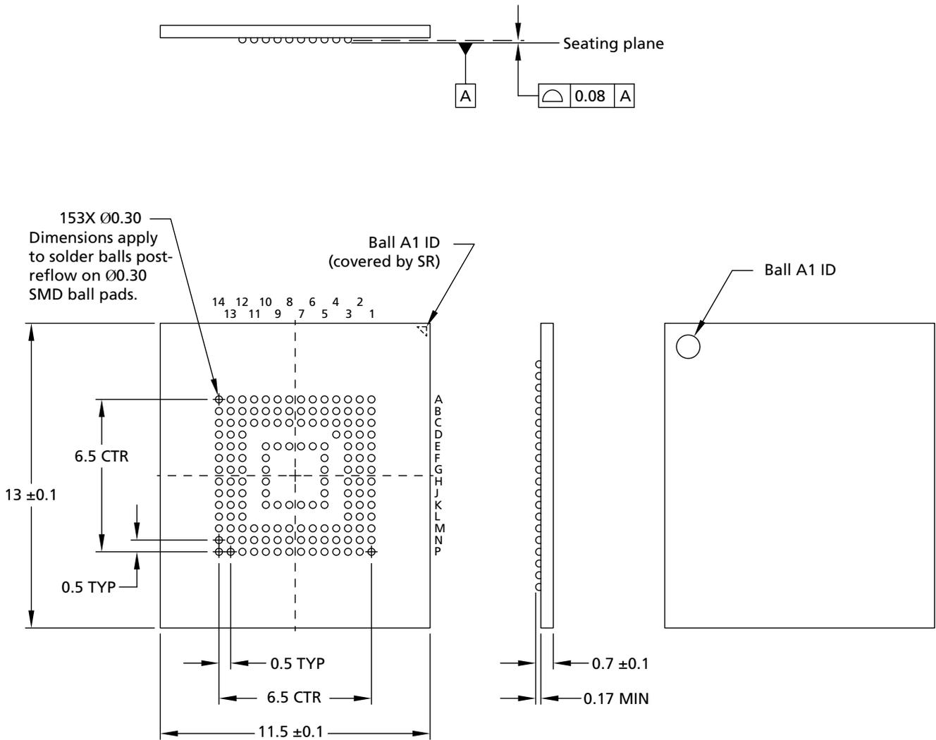
Note: 1. Dimensions are in millimeters.
