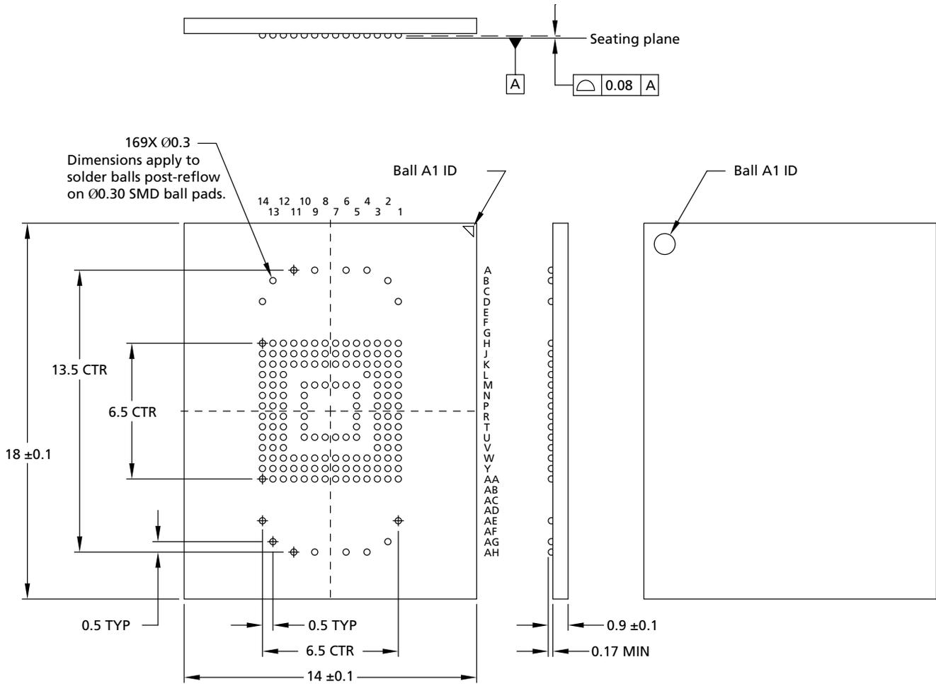
Note: 1. Dimensions are in millimeters.
