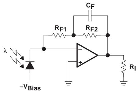
NOTE: Splitting the feedback resistor enables use of a larger, more manageable feedback capacitor.
