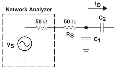
$$\frac{I_O}{V_S} = \frac{1}{2R_S \left(1 + \frac{C_1}{C_2}\right)} \quad (\text{above the pole frequency})$$
