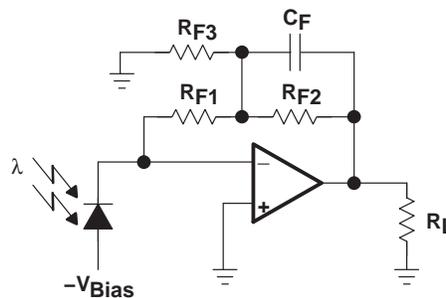
NOTE: A resistive T-network enables high transimpedance gain with reasonable resistor values.
