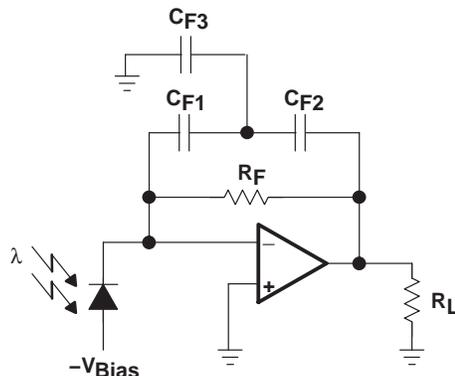
NOTE: A capacitive T-network enables fine control of the effective feedback capacitance using relatively large capacitor values.
