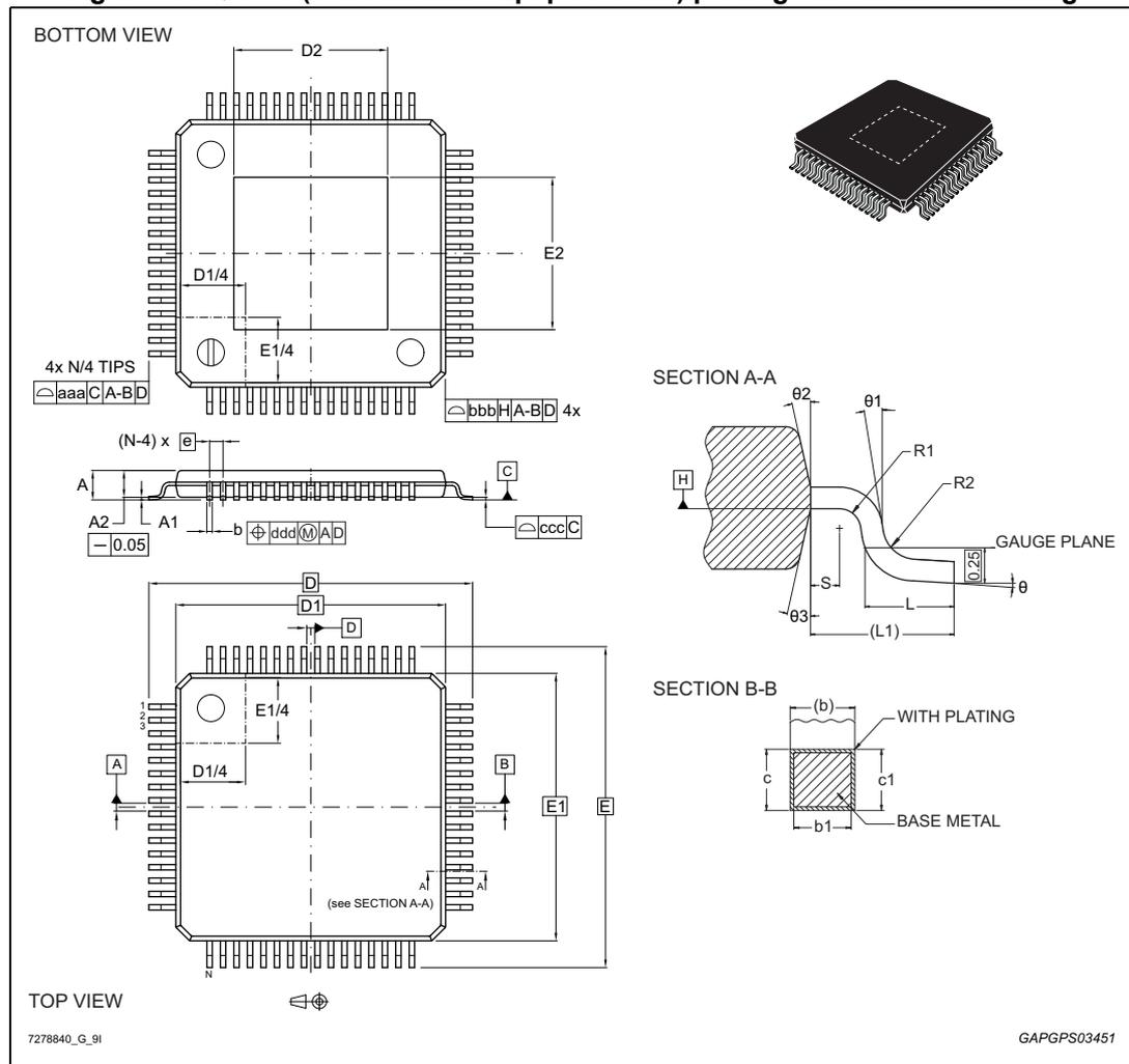
**Table 34. TQFP64 (10x10x1 mm exp. pad down) package mechanical data**
