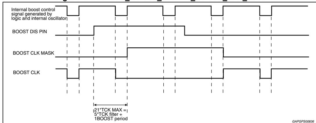
Figure 5. Case of T\_BOOST\_OFF > T\_BOOST\_OFF\_MAX
