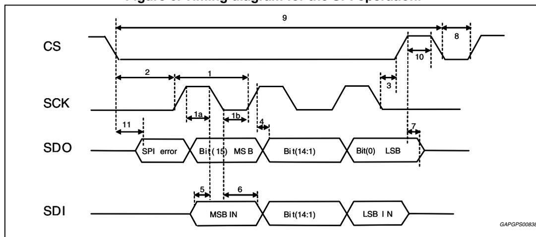
The SPI protocol integrates an internal check to add robustness to the communication: a writing attempt of a not allowed register, an incorrect parity frame or a wrong number of bits (different than 16) results in a "SPI error bit", that is available at SDO immediately after asserting CS the next time and before starting the SCK toggling.
