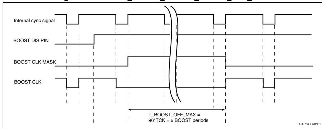
When `BST_DIS_EN` bit of `CMD2` SPI frame is set to 1 (refer to SPI mapping, [Table 20](#)), `BST_DIS` becomes a full-time control of the boost operation: the boost will be disabled as long as the `BST_DIS` pin is high. This implements a boost permanent disabler that can be used for different reasons, e.g. to allow more precise and less noisy measurements, to decrease power dissipation or current load on battery in all conditions when the boost is not strictly necessary.
