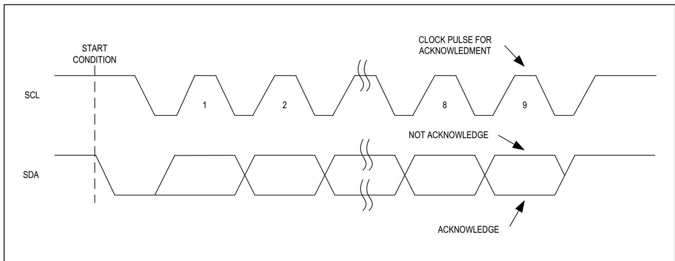
Figure 5. I<sup>2</sup>C Acknowledge Bit
