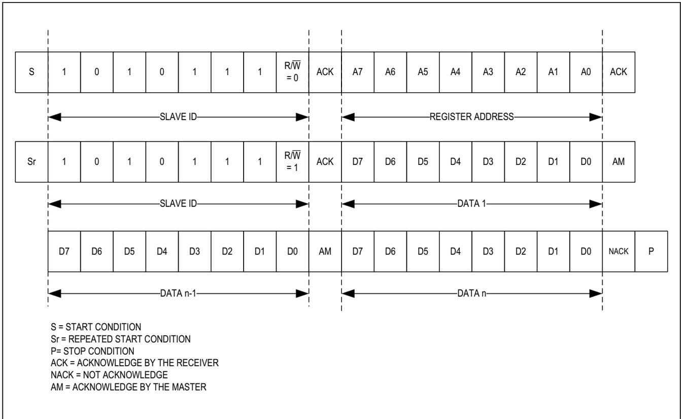
Figure 9. I<sup>2</sup>C Multi-Byte Read Transaction
