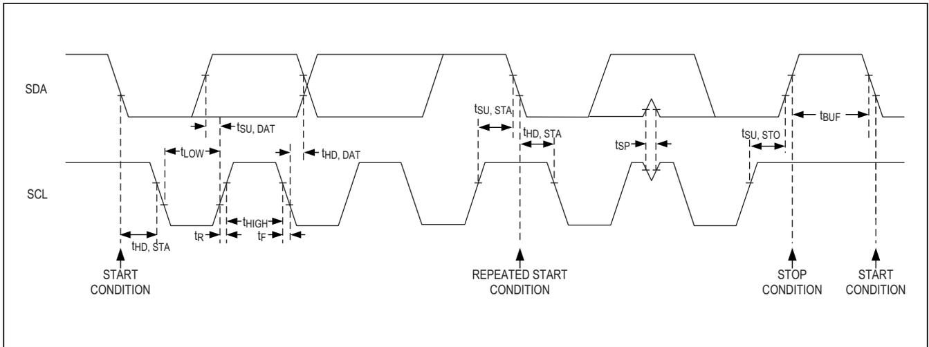
Figure 3. Detailed I<sup>2</sup>C Timing Diagram
