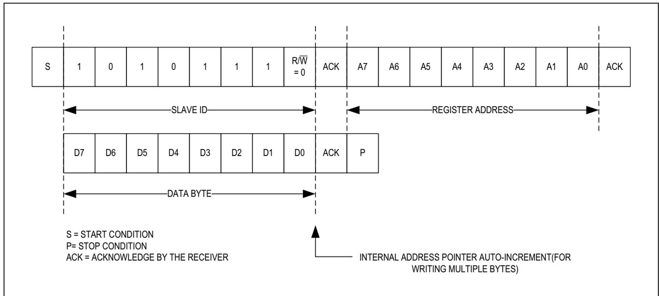
Figure 6. I<sup>2</sup>C Single Byte Write Transaction
