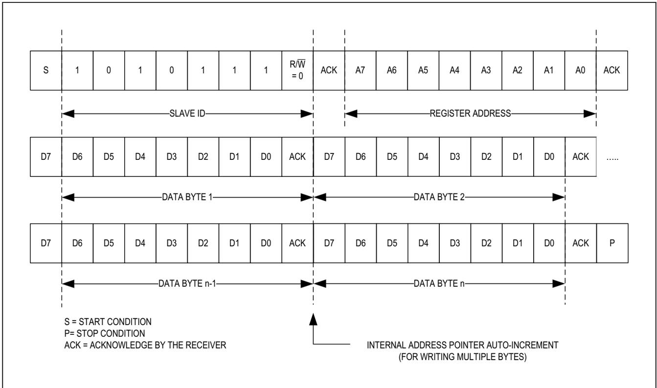
Figure 7. I<sup>2</sup>C Multi-Byte Write Transaction
