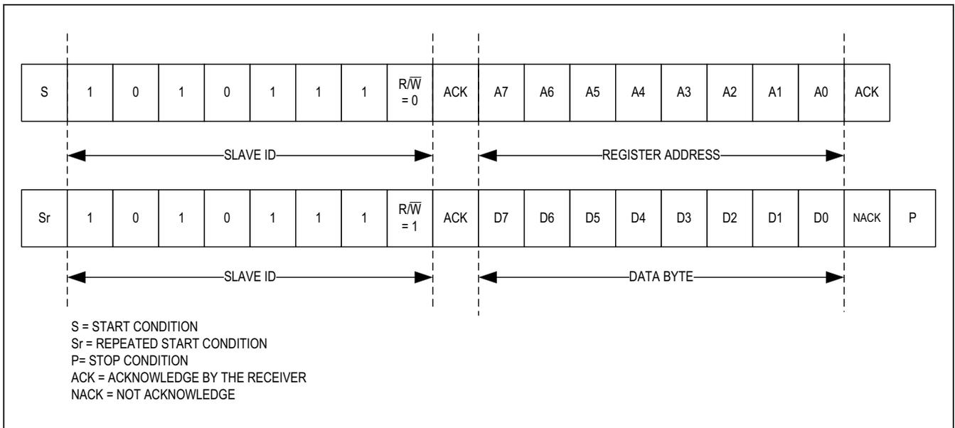
Figure 8. I<sup>2</sup>C Single Byte Read Transaction
