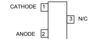
Pin 3 must left floating or connected to pin 2.
