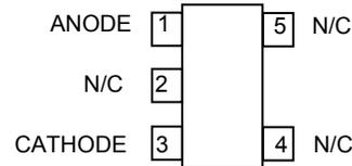
Pin 2 must be left floating or connected to pin 1
