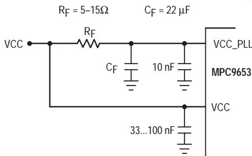
**Figure 3. VCC\_PLL Power Supply Filter**
