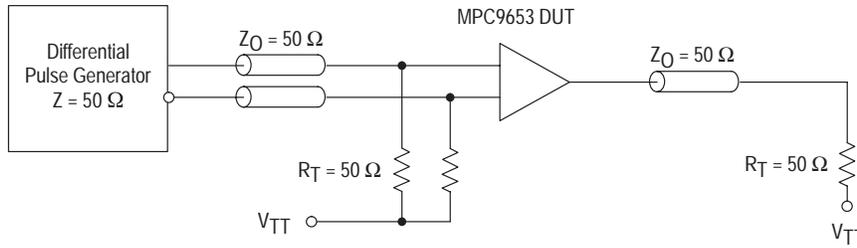
Figure 9. PCLK MPC9653 AC test reference
