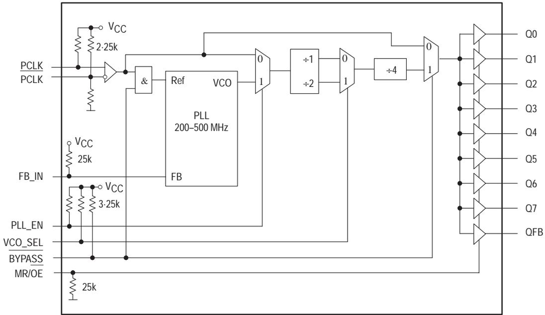
Figure 1. MPC9653 Logic Diagram
