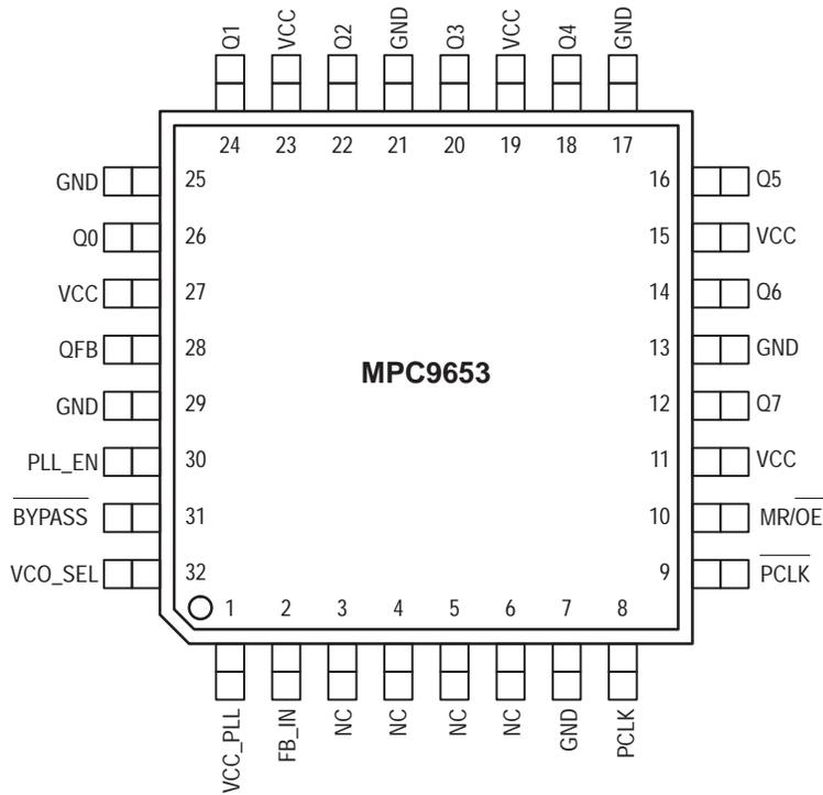
Figure 2. MPC9653 32-Lead Package Pinout (Top View)
