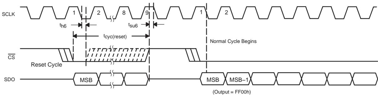
Figure 20. Critical Timing: Reset/Initialization Cycle (FS =1 for TLC4541)
