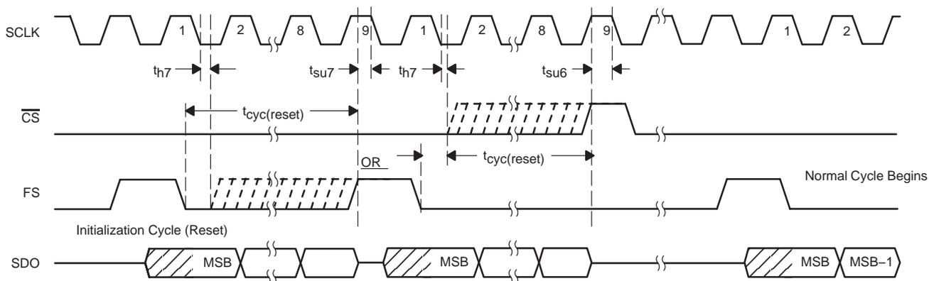
Figure 21. Critical Timing: Initialization Cycle (TLC4541 Only)
