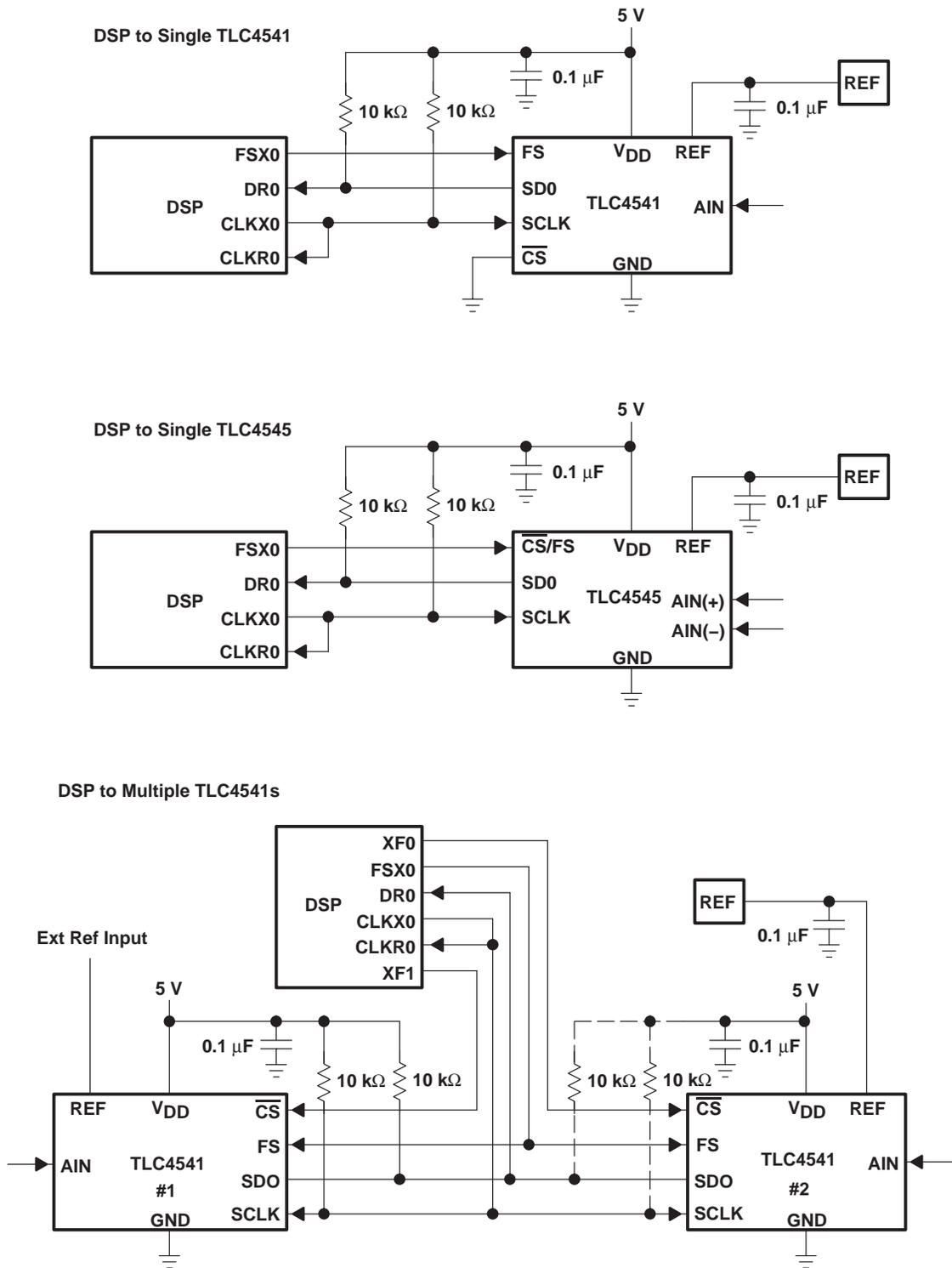
Figure 23. Typical ADC Interface to a TMS320 DSP
