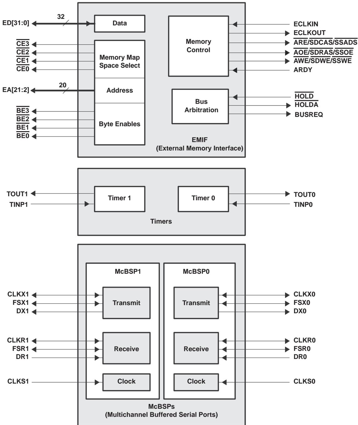
Figure 3. Peripheral Signals
