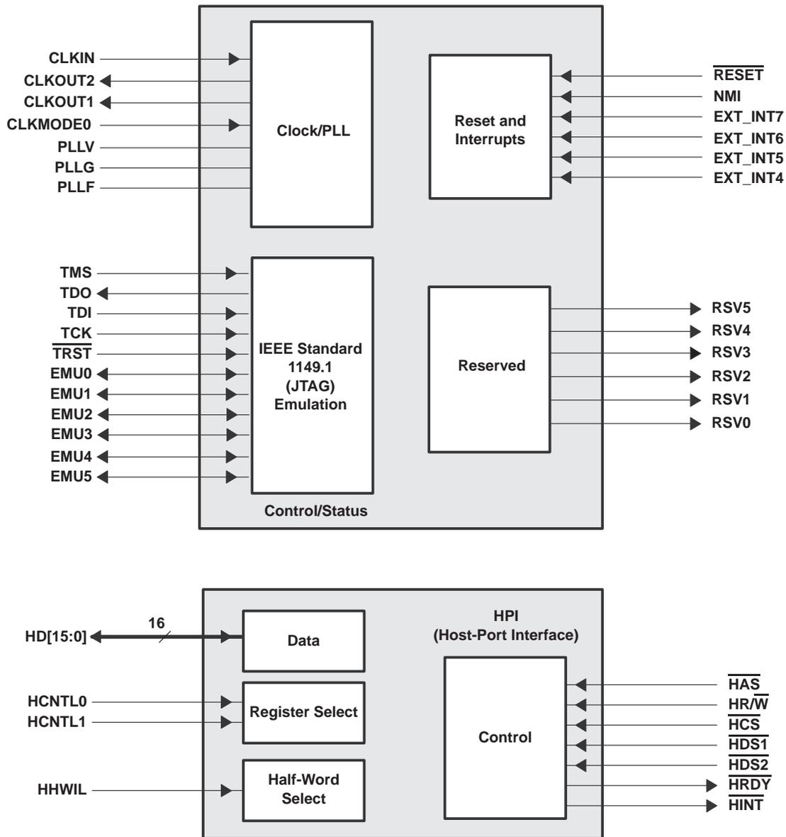
Figure 2. CPU (DSP Core) and Peripheral Signals
