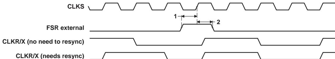
Figure 38. FSR Timing When GSYNC = 1
