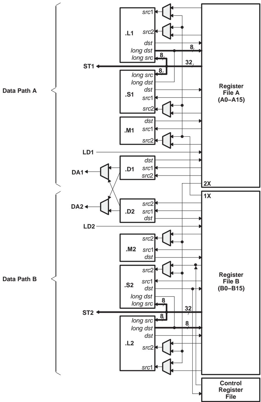
Figure 1. TMS320C62x™ CPU (DSP Core) Data Paths
