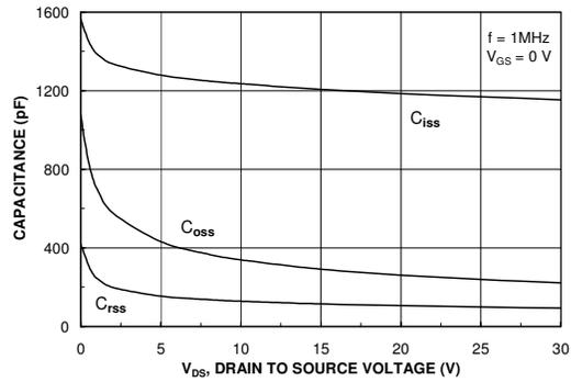
Figure 8. Capacitance Characteristics.
