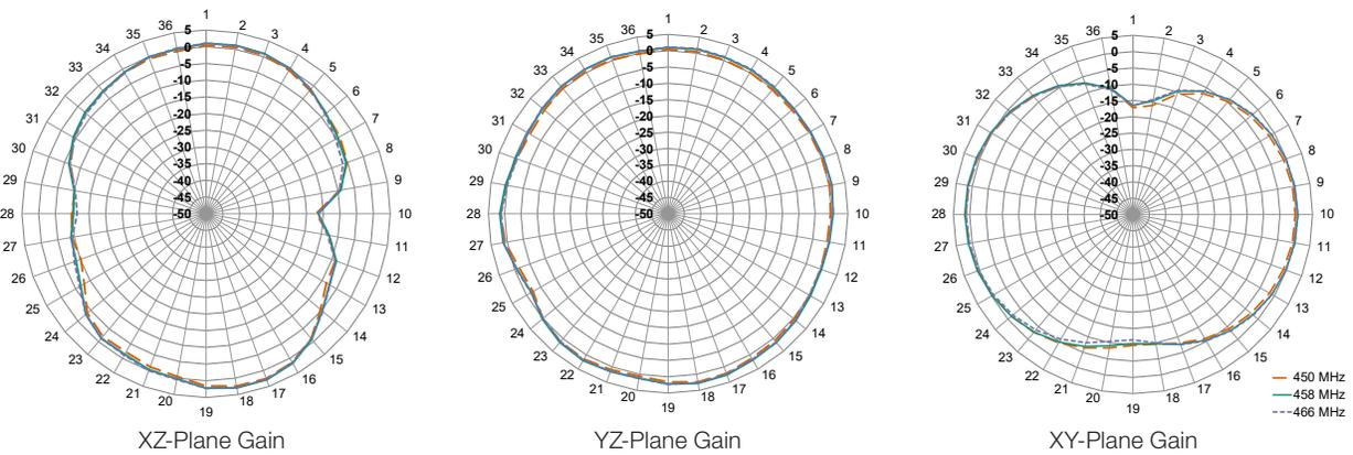
Figure8. Radiation Patterns for CW 450 MHz Antenna
