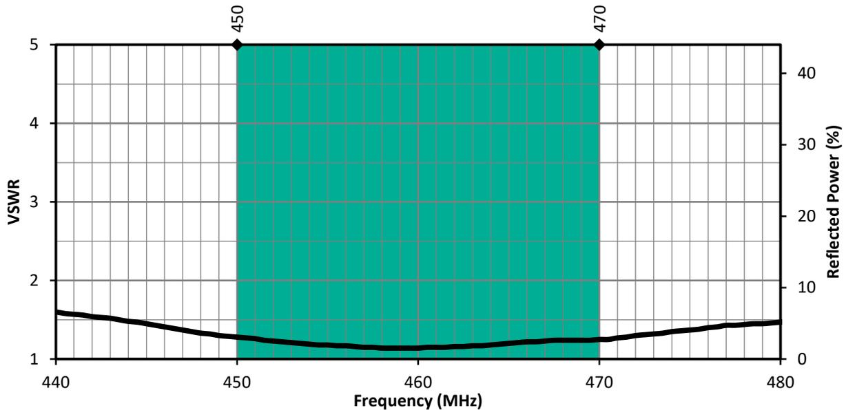
Figure 1. CW 450 MHz Antenna VSWR with Band Highlight
