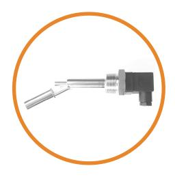
The SSF216 float switches are externally mounted horizontal switches. This switch has an extra-long reach to provide a solution for extra thick tank walls or for mounting through welded-on 1"NPT bosses.
