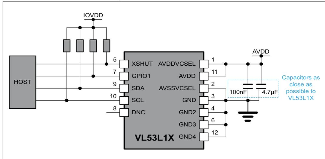
Note: Capacitors on external supply AVDD should be placed as close as possible to the AVDDVCSEL and AVSSVCSEL module pins.
