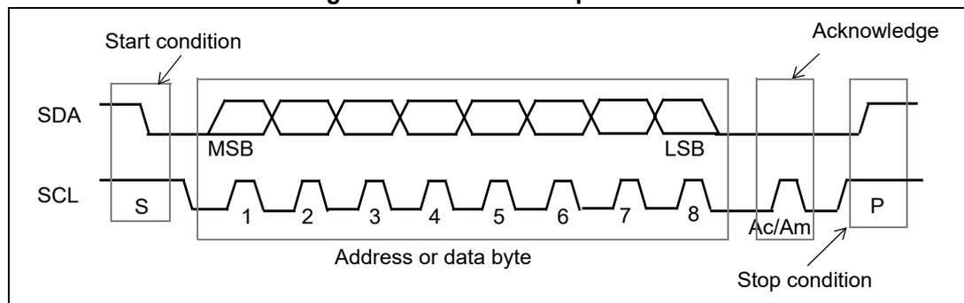
Information is packed in 8-bit packets (bytes) always followed by an acknowledge bit, Ac for VL53L1X acknowledge and Am for master acknowledge (host bus master). The internal data are produced by sampling SDA at a rising edge of SCL. The external data must be stable during the high period of SCL. The exceptions to this are start (S) or stop (P) conditions when SDA falls or rises respectively, while SCL is high.
