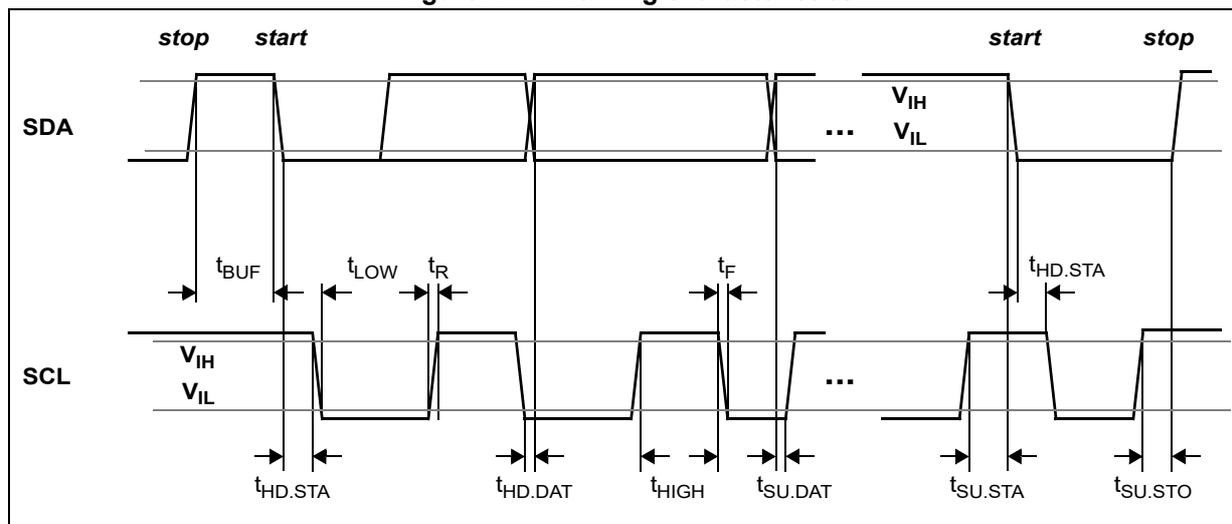
All timings are measured from either V<sub>IL</sub> or V<sub>IH</sub>.
