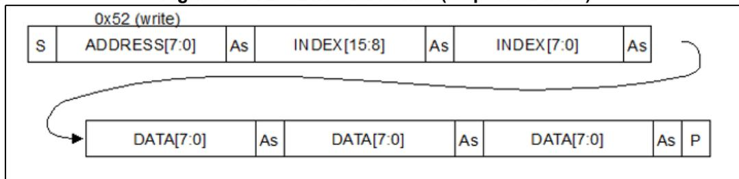
Figure 16. VL53L1X data format (sequential read)
