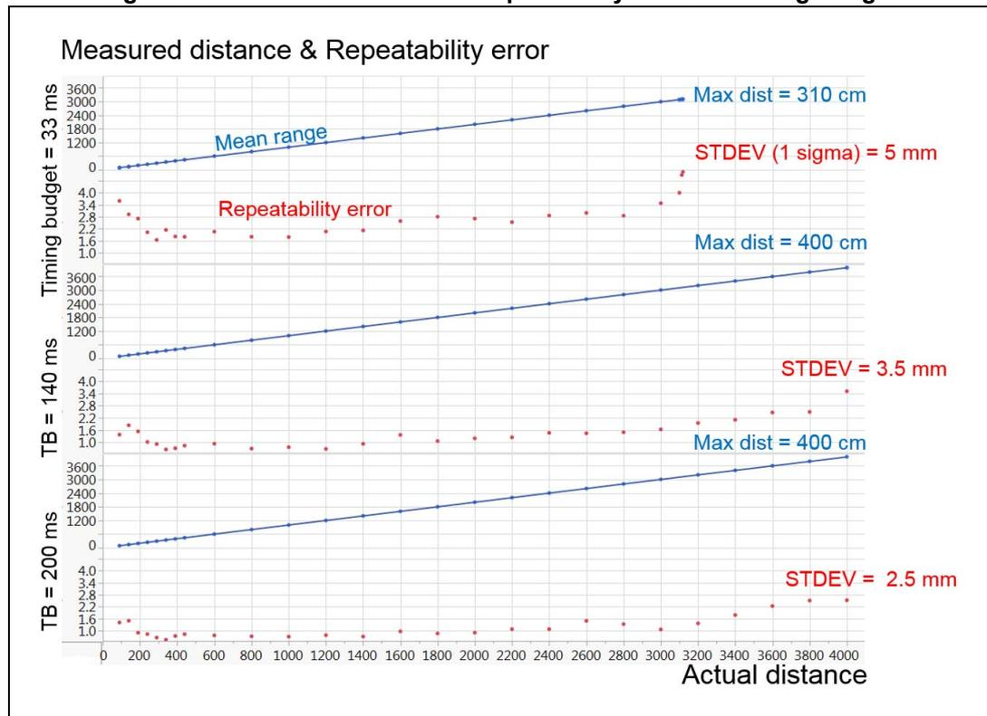
Test conditions: timing budget = 33 ms, 140 ms, 200 ms, grey target 54%, ambient light = dark.
