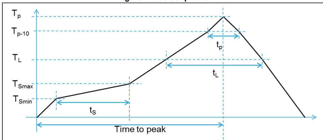
Note: Temperature mentioned in [Table 18](#) is measured at the top of the VL53L1X package.
