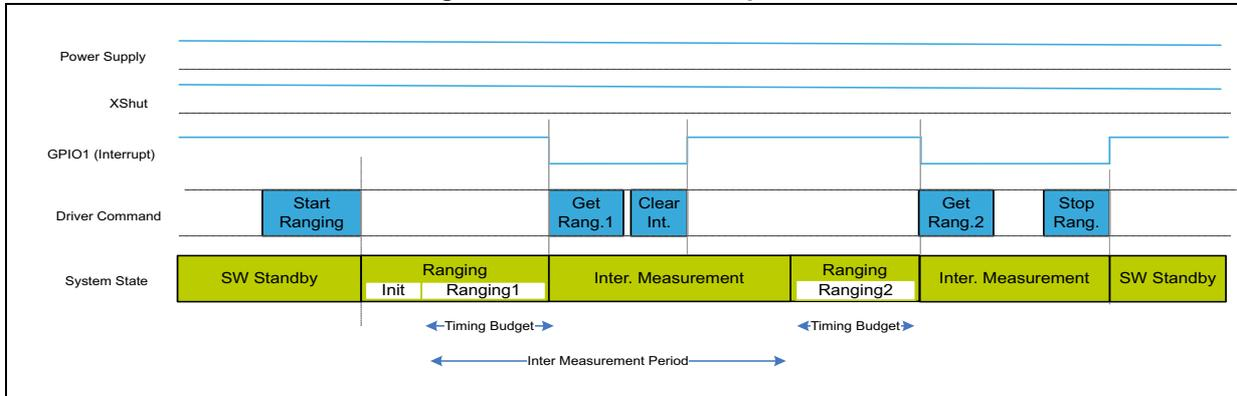
*Note:* Timing budget and inter measurement timings are the parameters set by the user, using a dedicated driver function.
