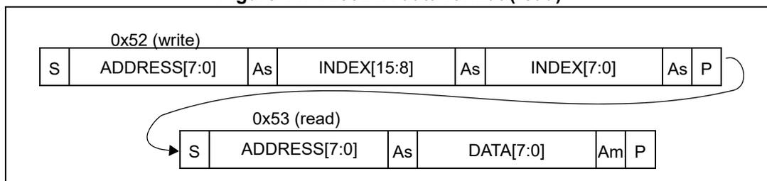
At the end of each byte, in both read and write message sequences, an acknowledge is issued by the receiving device (that is, the VL53L1X for a write and the host for a read).
