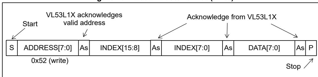
As data are received by the slave, they are written bit-by-bit to a serial/parallel register. After each data byte has been received by the slave, an acknowledge is generated, the data are then stored in the internal register addressed by the current index.
