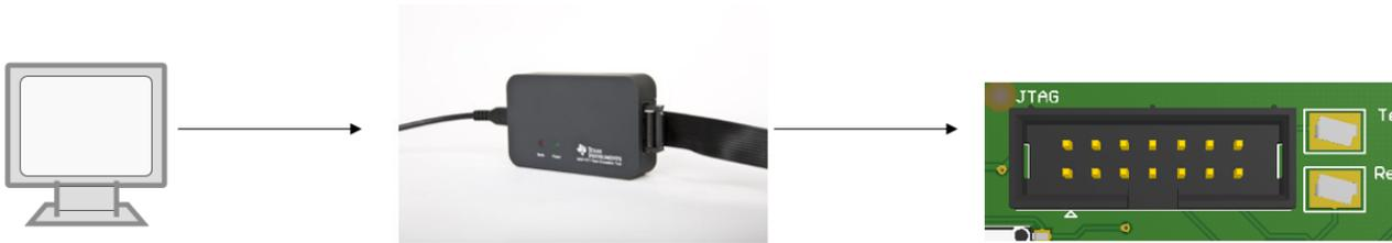
**Figure 19. MSP-FET and TIDA-01373 System Diagram**
