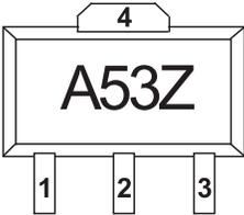
Alternate marking SGA5489Z on line 1 with Trace Code on line 2.
