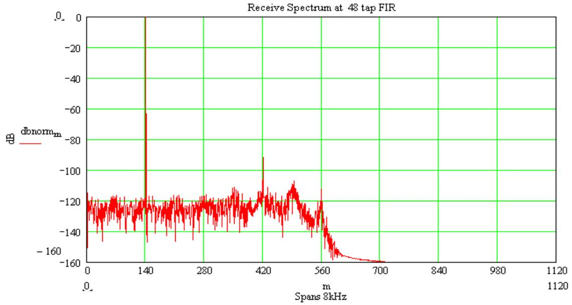
**Figure 8: RXD Spectrum of 1 kHz Tone**
