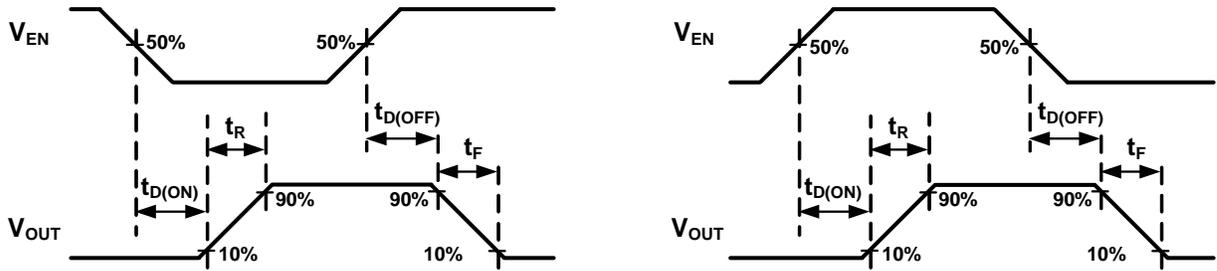
Figure 1. Voltage Waveforms: AP2162A (Left), AP2172A (Right)
