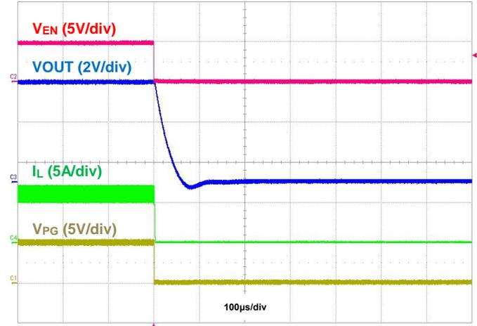
Figure 10. Shutdown Using EN, IOU = 6A
