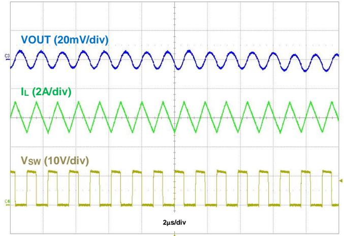
Figure 19. Output Voltage Ripple,  $I_{\text{OUT}} = 6\text{A}$
