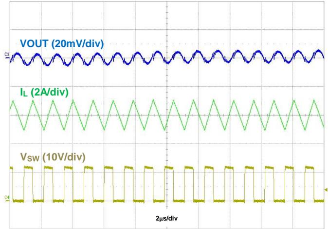
Figure 41. Output Voltage Ripple,  $I_{OUT} = 6\text{A}$
