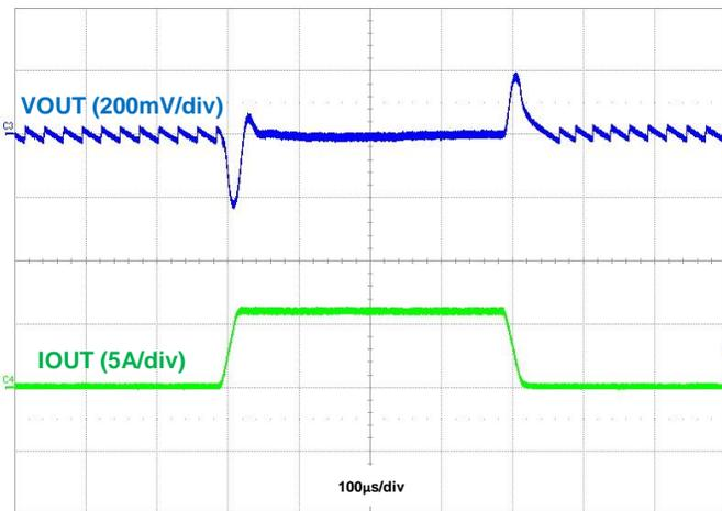
Figure 22. Load Transient,  $I_{\text{OUT}} = 50\text{mA}$  to  $6\text{A}$  to  $50\text{mA}$
