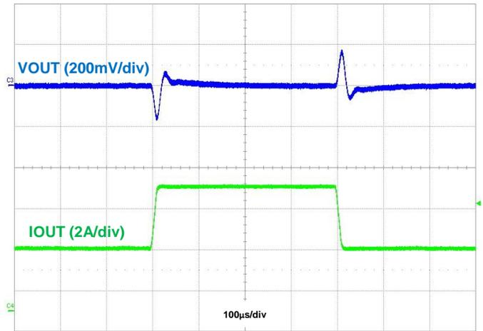
Figure 21. Load Transient,  $I_{\text{OUT}} = 3\text{A}$  to  $6\text{A}$  to  $3\text{A}$
