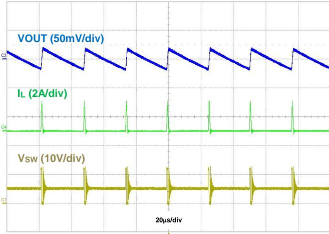
Figure 29. Output Voltage Ripple,  $I_{OUT} = 50\text{mA}$
