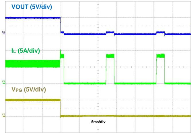
Figure 11. Output Short Protection, IOU = 6A
