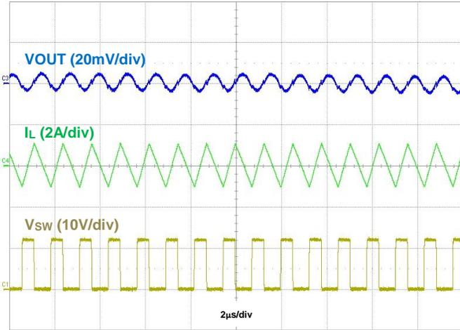
Figure 40. Output Voltage Ripple,  $I_{OUT} = 50\text{mA}$
