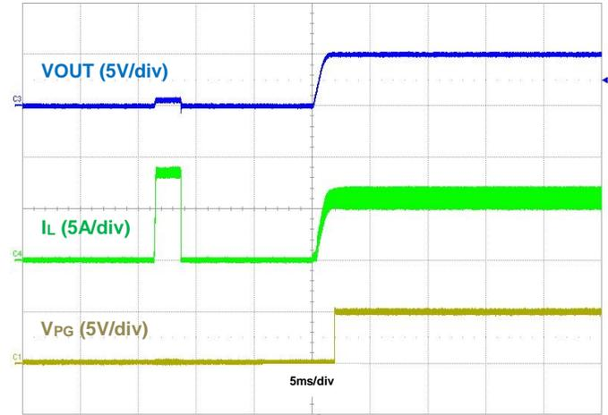
Figure 12. Output Short Recovery, IOU = 6A
