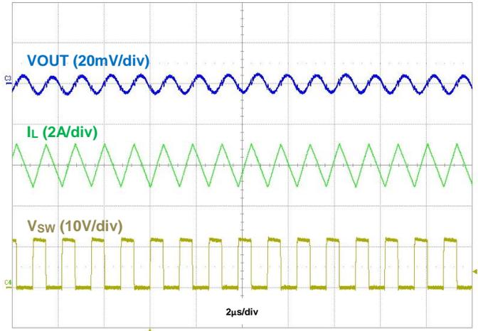
Figure 30. Output Voltage Ripple,  $I_{OUT} = 6\text{A}$
