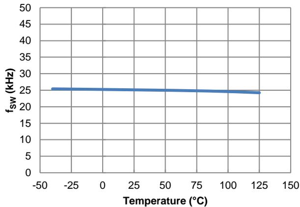
Figure 27.  $f_{sw}$  vs. Temperature,  $I_{OUT} = 0\text{A}$
