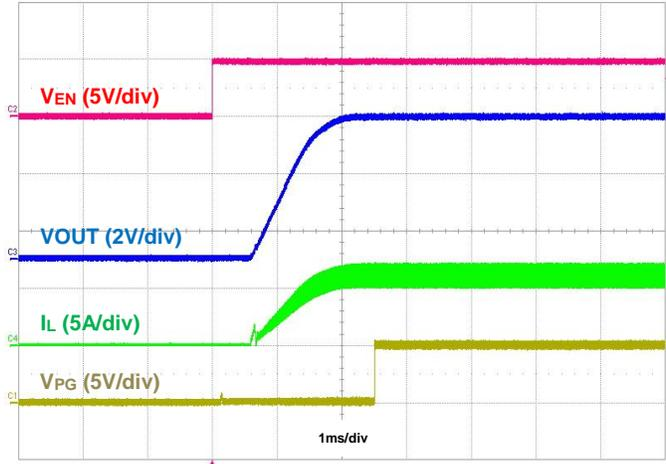
Figure 9. Startup Using EN, IOU = 6A
