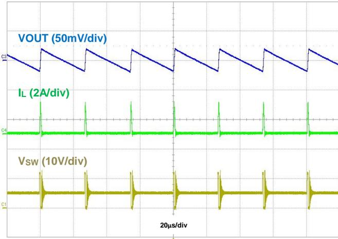
Figure 18. Output Voltage Ripple,  $I_{\text{OUT}} = 50\text{mA}$
