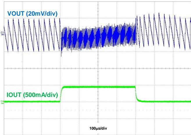
Figure 20. Load Transient,  $I_{\text{OUT}} = 50\text{mA}$  to  $500\text{mA}$  to  $50\text{mA}$
