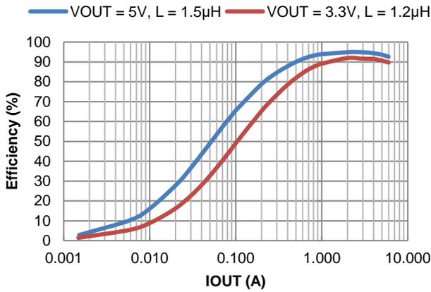
Figure 34. Efficiency vs. Output Current,  $V_{IN} = 12\text{V}$
