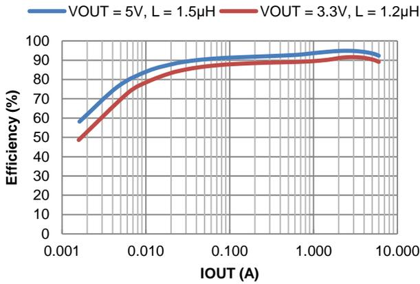
Figure 13. Efficiency vs. Output Current,  $V_{IN} = 12\text{V}$
