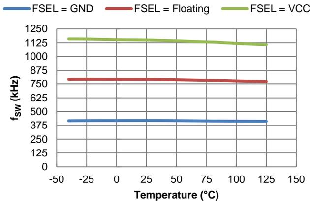
Figure 38.  $f_{sw}$  vs. Temperature,  $I_{OUT} = 0\text{A}$
