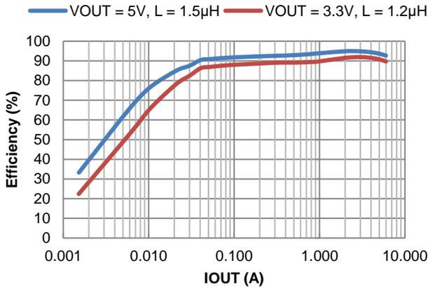
Figure 23. Efficiency vs. Output Current,  $V_{IN} = 12\text{V}$
