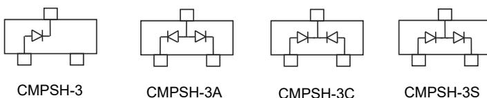
**350mW 30Volt Switching Diode**
