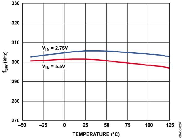
Figure 20. Switching Frequency vs. Temperature,  $f_{sw} = 300 \text{ kHz}$
