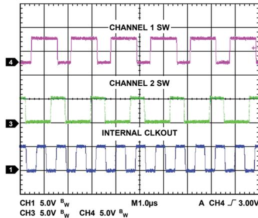
Figure 67. CLKOUT Waveforms
