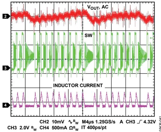
Figure 41. Pulse Skip Mode, 110 mA Load
