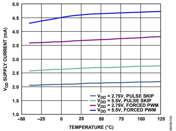
Figure 34. V<sub>DD</sub> Supply Current vs. Temperature, Channel 1: V<sub>OUT1</sub> = 1.5 V, Channel 2: V<sub>OUT2</sub> = 0.8 V, f<sub>SW</sub> = 1.2 MHz
