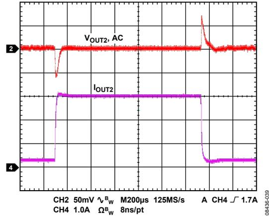
Figure 39. Load Transient Response in Pulse Skip Mode, Channel 2: 0.3 A to 3 A Load Step,  $V_{IN} = 3.3\text{ V}$ ,  $V_{OUT} = 1.2\text{ V}$ ,  $f_{SW} = 1.2\text{ MHz}$  (See Table 12 for the Circuit Details)
