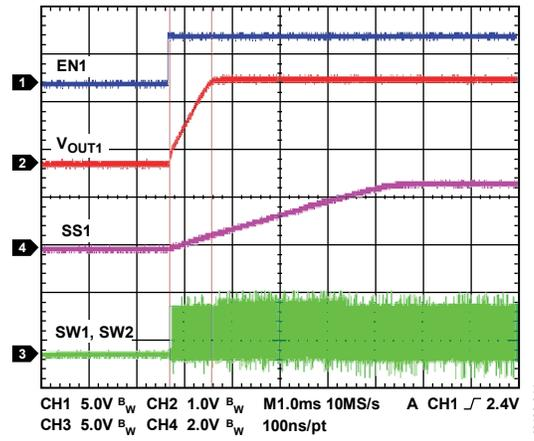
Figure 44. Soft Start, Channel 1:  $V_{OUT} = 1.8V$ ,  $C_{SS1} = 10nF$
