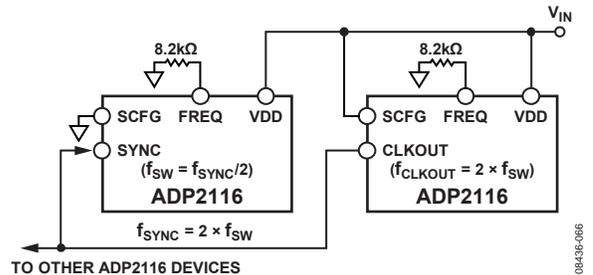
Figure 66. ADP2116 to Synchronize with Another ADP2116 (f<sub>sw</sub> = 600 kHz; the SCFG Pin of the Master Is Tied to VDD)
