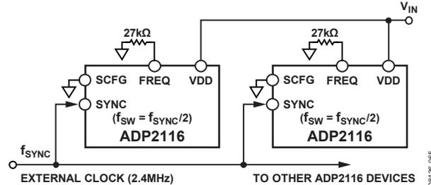
Figure 65. Synchronization with External Clock (f<sub>sw</sub> = 1.2 MHz)
