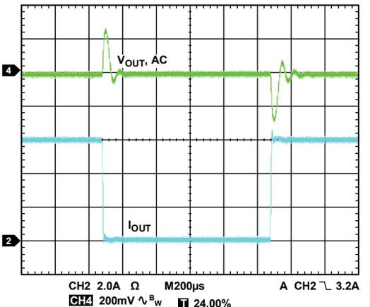
Figure 37. Load Transient Response in Forced PWM Mode, Combined Output: 0 A to 6 A Load Step,  $V_{IN} = 5\text{ V}$ ,  $V_{OUT} = 3.3\text{ V}$ ,  $f_{SW} = 600\text{ kHz}$  (See Table 12 for the Circuit Details)
