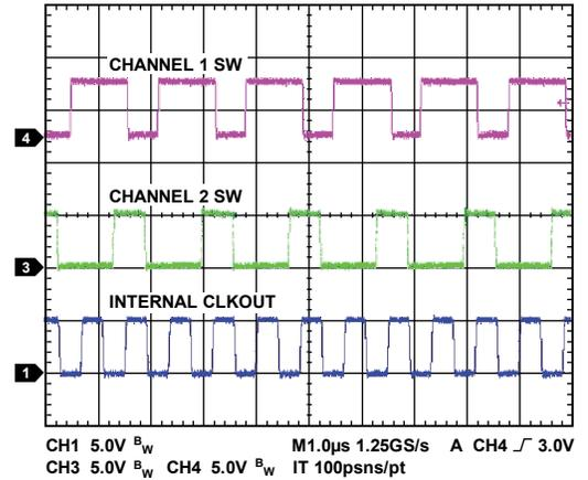
Figure 51. Internal Clock Output,  $f_{SW} = 600kHz$ ,  $f_{CLKOUT} = 1.2MHz$
