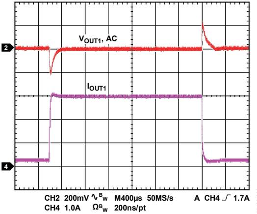
Figure 36. Load Transient Response in Pulse Skip Mode, Channel 1: 0.3 A to 3 A Load Step,  $V_{IN} = 5\text{ V}$ ,  $V_{OUT} = 3.3\text{ V}$ ,  $f_{SW} = 300\text{ kHz}$  (See Table 12 for the Circuit Details)
