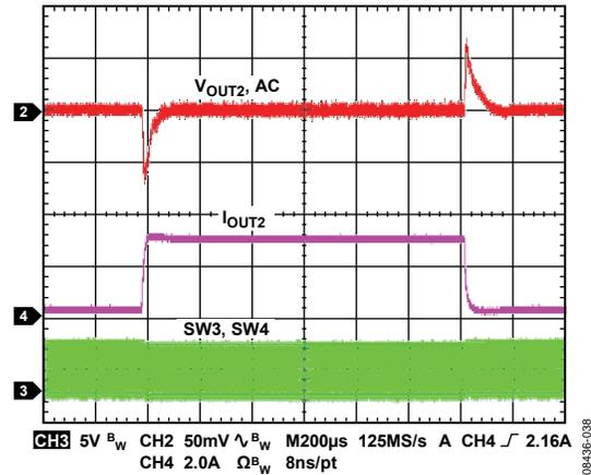
Figure 38. Load Transient Response in Pulse Skip Mode, Channel 2: 0.3 A to 3 A Load Step,  $V_{IN} = 5\text{ V}$ ,  $V_{OUT} = 1.2\text{ V}$ ,  $f_{SW} = 600\text{ kHz}$  (See Table 12 for the Circuit Details)
