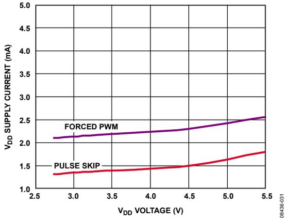
Figure 31. V<sub>DD</sub> Supply Current, No Load, Channel 1: V<sub>OUT1</sub> = 1.5 V, Channel 2: Off, f<sub>SW</sub> = 1.2 MHz
