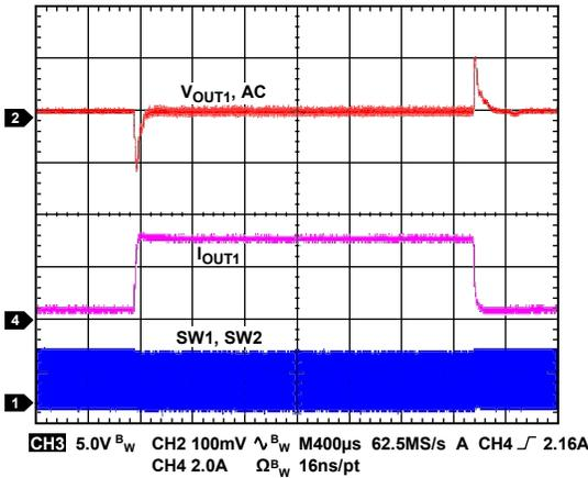
Figure 35. Load Transient Response in Pulse Skip Mode, Channel 1: 0.3 A to 3 A Load Step,  $V_{IN} = 5\text{ V}$ ,  $V_{OUT} = 2.5\text{ V}$ ,  $f_{SW} = 600\text{ kHz}$  (See Table 12 for the Circuit Details)
