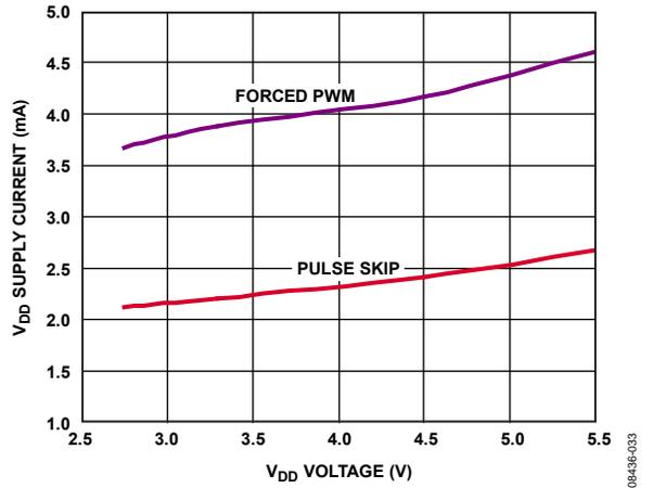
Figure 33. V<sub>DD</sub> Supply Current, No Load, Channel 1: V<sub>OUT1</sub> = 1.5 V, Channel 2: V<sub>OUT2</sub> = 0.8 V, f<sub>SW</sub> = 1.2 MHz
