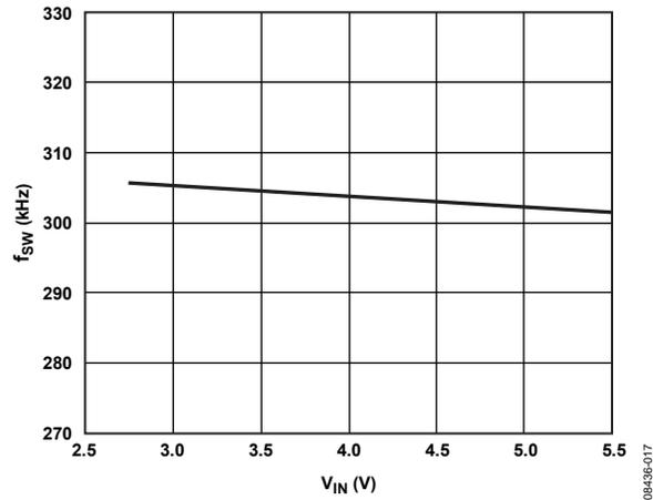
Figure 17. Switching Frequency vs. Input Voltage, f<sub>SW</sub> = 300 kHz
