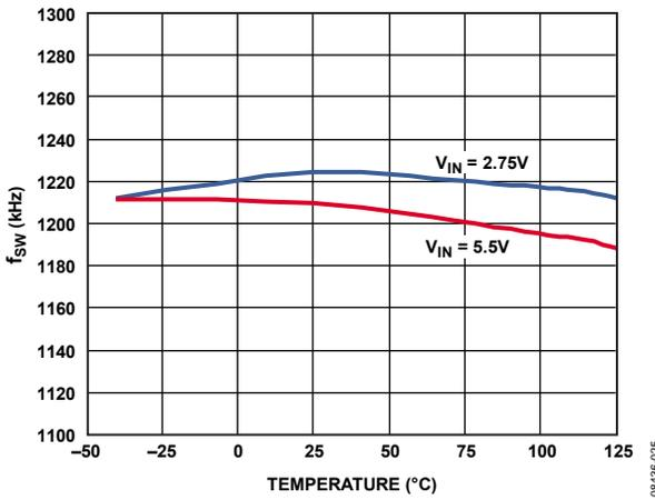
Figure 25. Switching Frequency vs. Temperature,  $f_{sw} = 1.2 \text{ MHz}$
