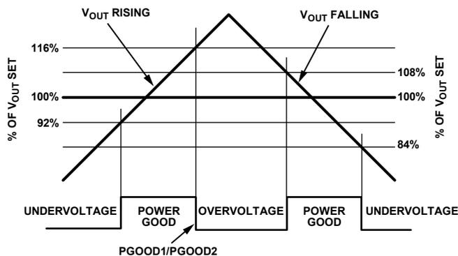
Figure 60. PGOOD1/PGOOD2 Thresholds
