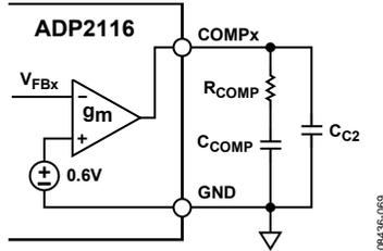
Figure 69. Compensation Components
