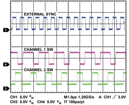
Figure 50. External Synchronization,  $f_{SYNC} = 1.5MHz$ ,  $f_{SW} = 750kHz$
