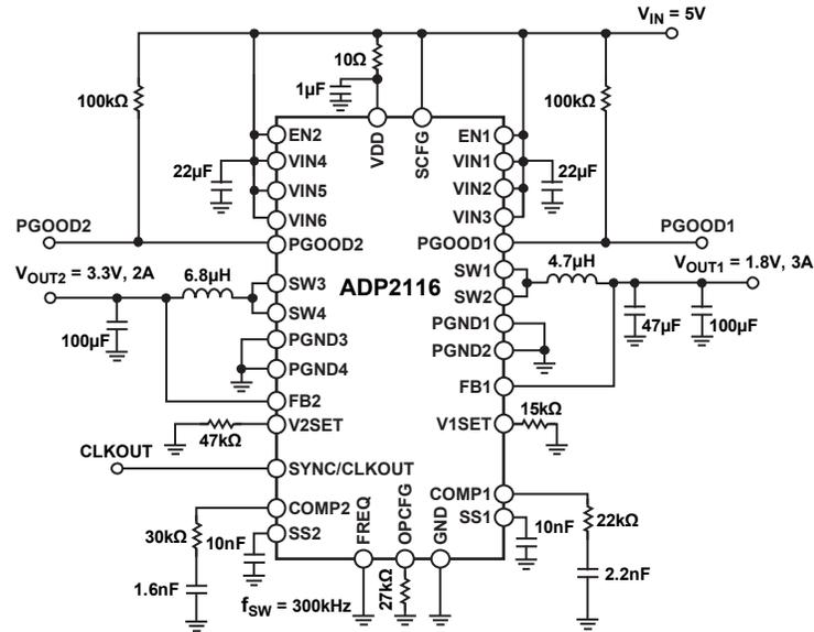
Figure 73. Application Circuit for 3 A/2 A Outputs
