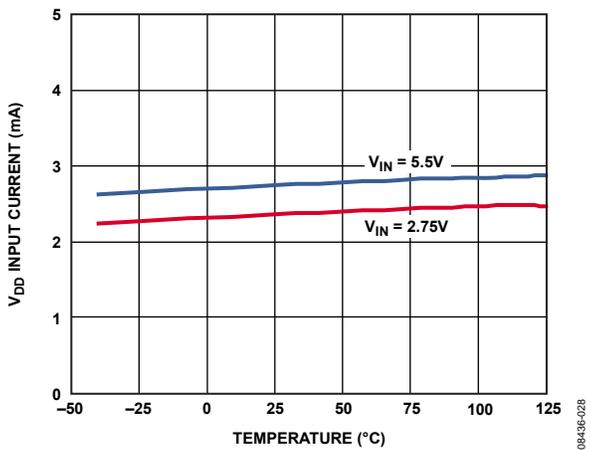
Figure 28. V<sub>DD</sub> Input Current vs. Temperature, Not Switching
