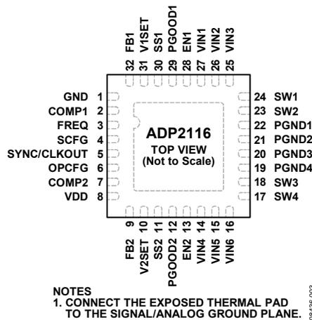
Figure 3. Pin Configuration
