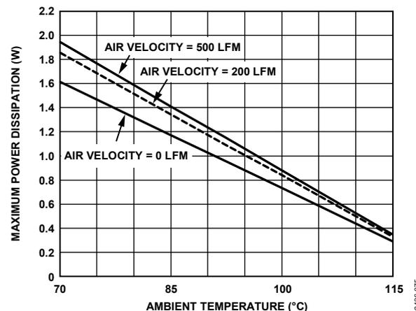
Figure 75. Power Dissipation Derating (JEDEC 1S2P Board)
