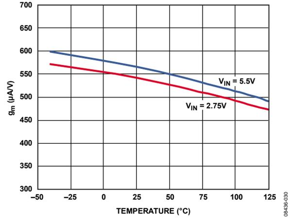
Figure 30. g<sub>m</sub> vs. Temperature
