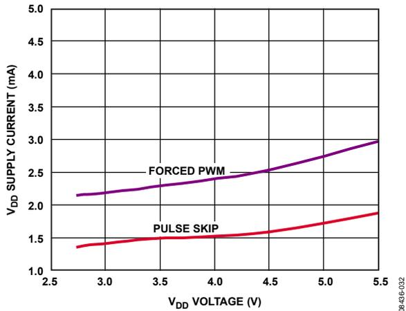
Figure 32. V<sub>DD</sub> Supply Current, No Load, Channel 2: V<sub>OUT2</sub> = 0.8 V, Channel 1: Off, f<sub>SW</sub> = 1.2 MHz
