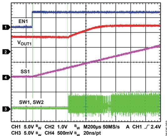
Figure 59. Soft Start with a Precharged Output
