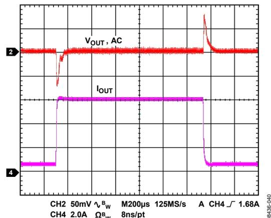
Figure 40. Load Transient Response in Forced PWM Mode, Combined Output: 0.6 A to 6 A Load Step,  $V_{IN} = 5\text{ V}$ ,  $V_{OUT} = 1.2\text{ V}$ ,  $f_{SW} = 600\text{ kHz}$  (See Table 12 for the Circuit Details)
