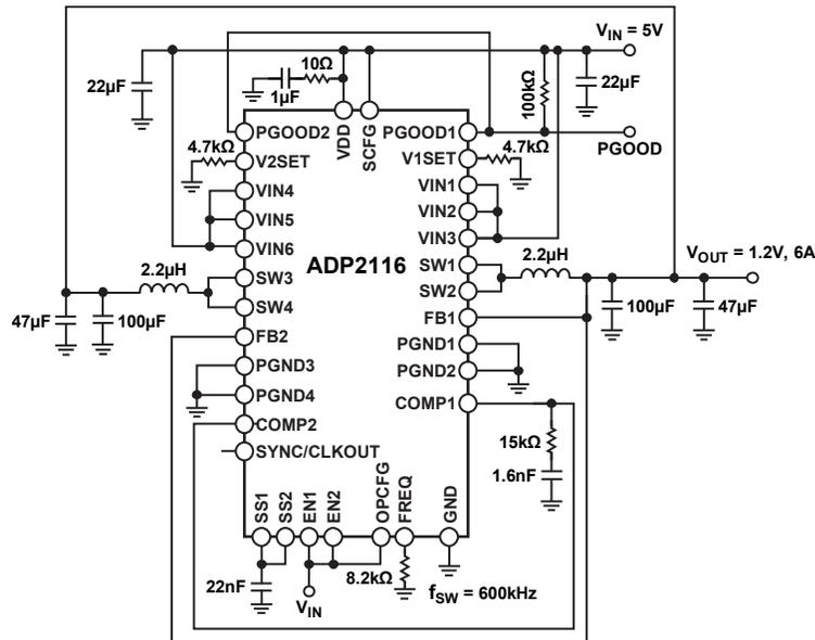
Figure 72. Application Circuit for a Single 6 A Output
