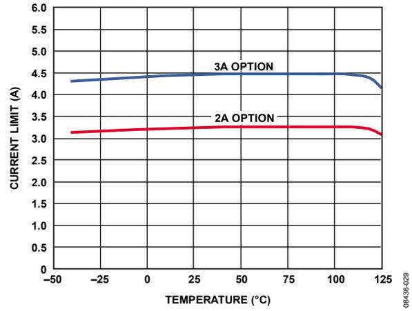
Figure 29. Peak Current Limit vs. Temperature, V<sub>IN</sub> = 5V
