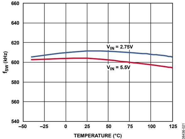
Figure 21. Switching Frequency vs. Temperature,  $f_{sw} = 600 \text{ kHz}$
