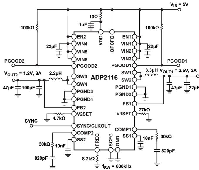
Figure 71. Application Circuit for 3 A/3 A Outputs
