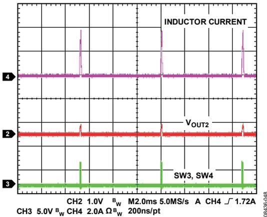
Figure 48. Hiccup Mode,  $f_{SW} = 600kHz$ , 6.8ms Hiccup Cycle
