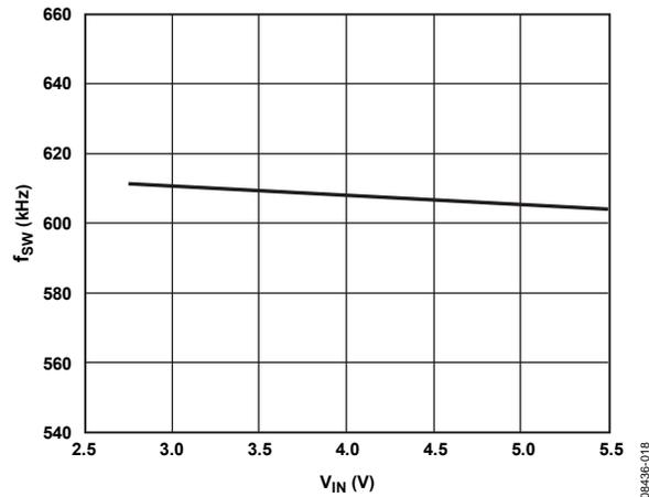
Figure 18. Switching Frequency vs. Input Voltage, f<sub>SW</sub> = 600 kHz
