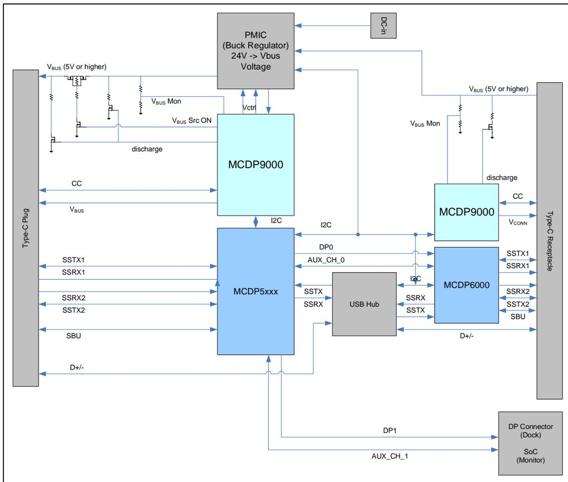
Figure 3 shows a typical use case of the MCDP9000 with a Kinetics’ DisplayPort converter product in an AV adapter. The AV adapter is going to use  $V_{BUS}$  line for its own power supply. 5V / 3A power profile should suffice for this application. Therefore, minimum BOM will be required in this use case. Because this
