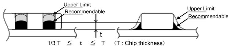
Accordingly increasing the solder volume, the mechanical stress to product is also increased. Excessive solder volume may cause the failure of mechanical or electrical performance.
