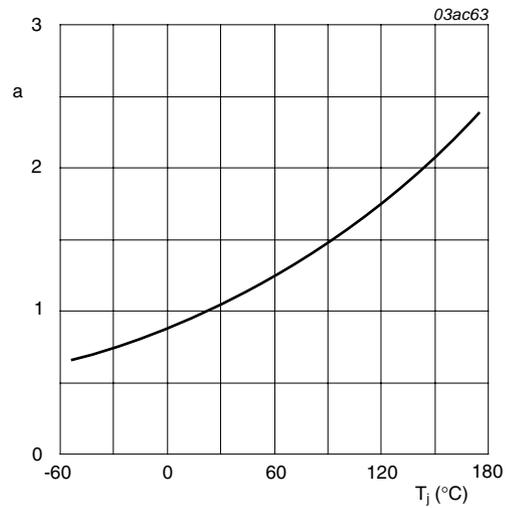
$$a = \frac{R_{DSon}}{R_{DSon(25^{\circ}C)}}$$
