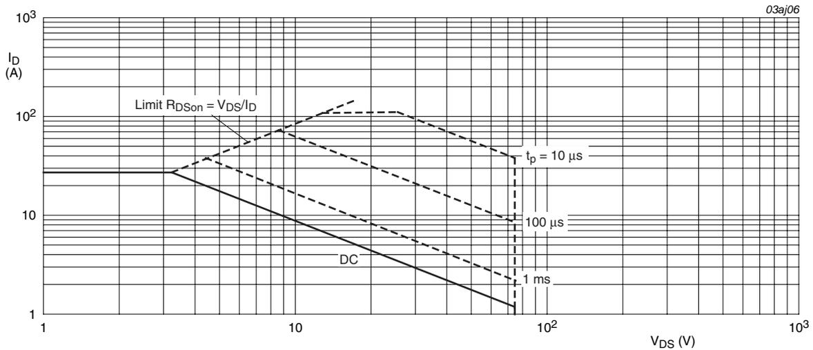
$T_{mb} = 25^\circ\text{C}; I_{DM}$  is single pulse;  $V_{GS} = 11\text{V}$
