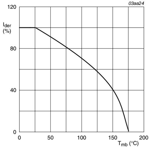
$$I_{der} = \frac{I_D}{I_{D(25^\circ\text{C})}} \times 100\%$$
