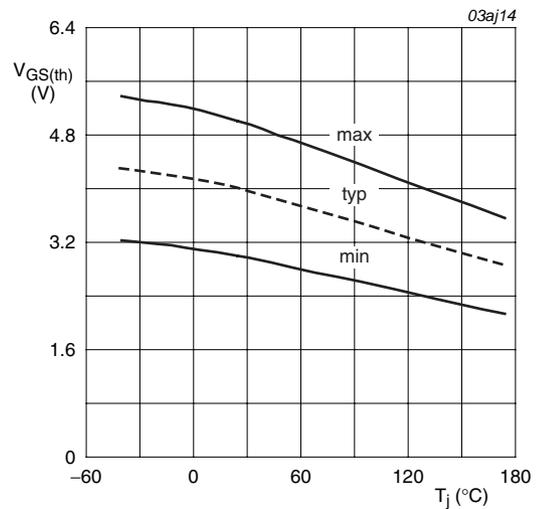
$I_D = 2\text{mA}; V_{DS} = V_{GS}$
