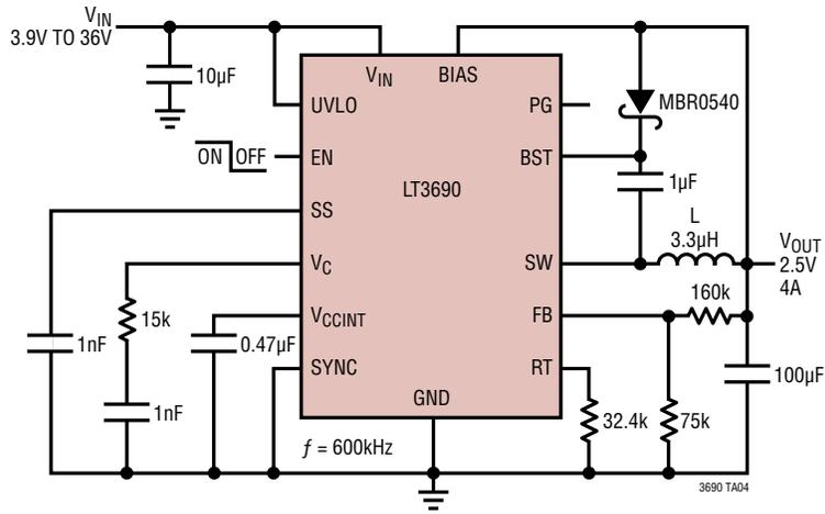
(FIXED FREQUENCY AT  $V_{IN} < 21V$ )
