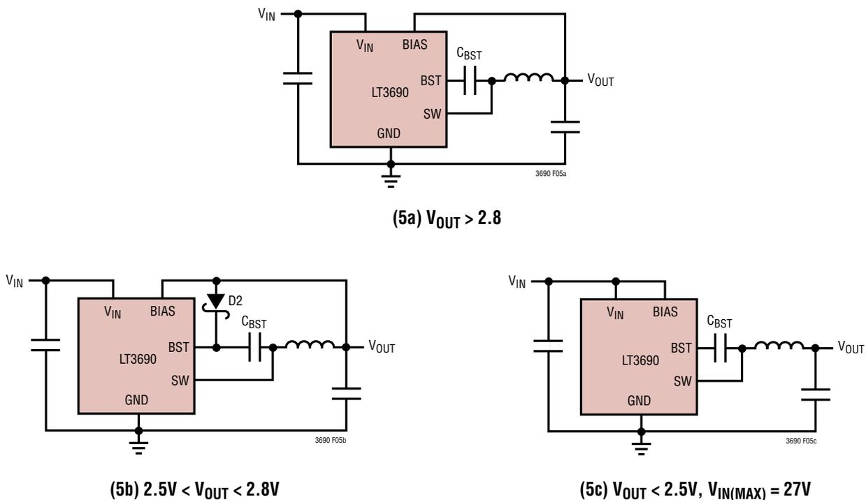
Figure 5. Three Circuits for Generating the Boost Voltage
