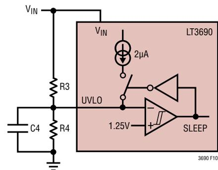
Figure 10. Undervoltage Lockout
