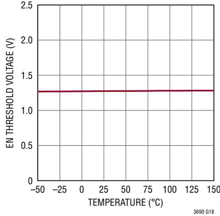
**UVLO Threshold Voltage vs Temperature**
