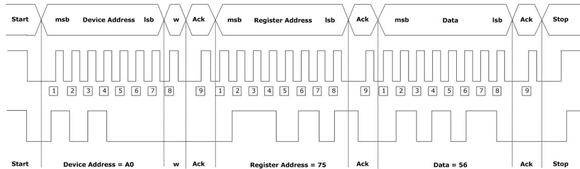
**Figure 11 • Read Cycle Diagram**
