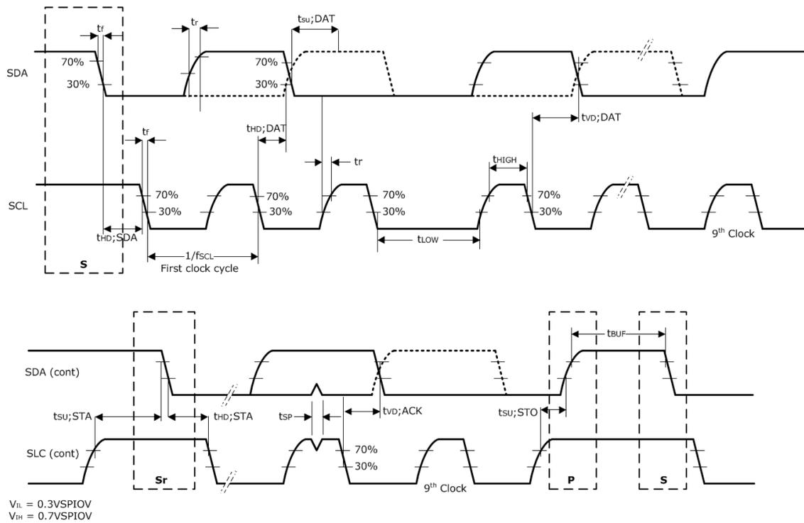
**Figure 9 • Timing Definition for HS-Mode Devices on the I2C Port**
