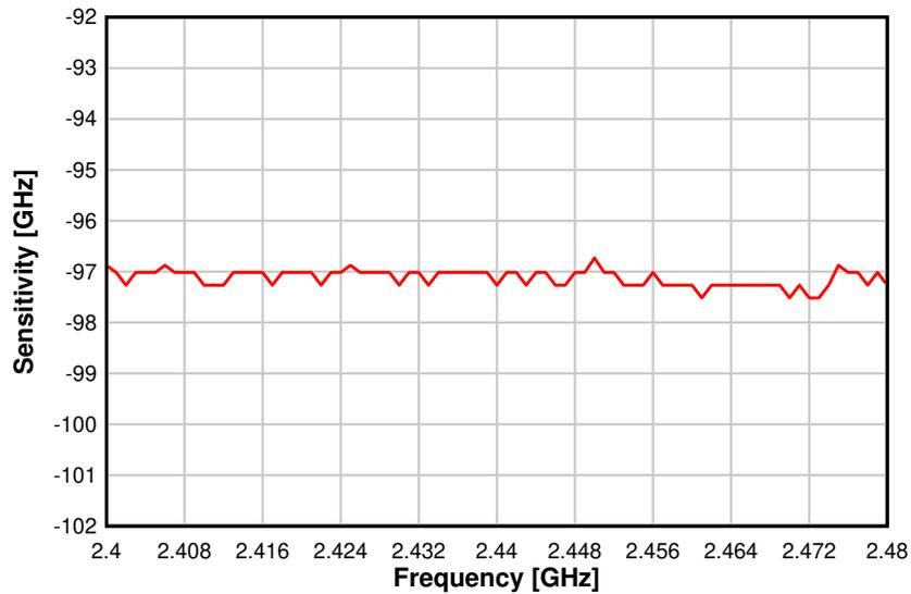
**Figure 8-11. Sensitivity vs. Frequency (BLE 1 Mbps, 2.44 GHz)**
