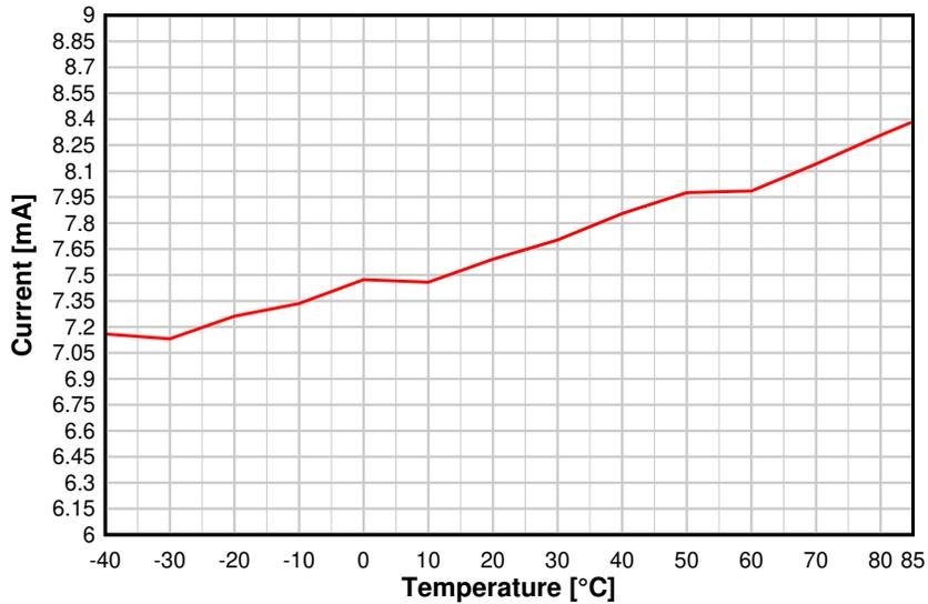
Figure 8-9. TX Current vs. Temperature (BLE 1 Mbps, 2.44 GHz)
