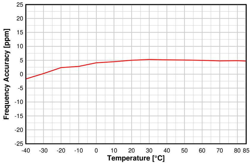
**Figure 8-24. Compensated Frequency Accuracy vs. Temperature (2.44 GHz)**
