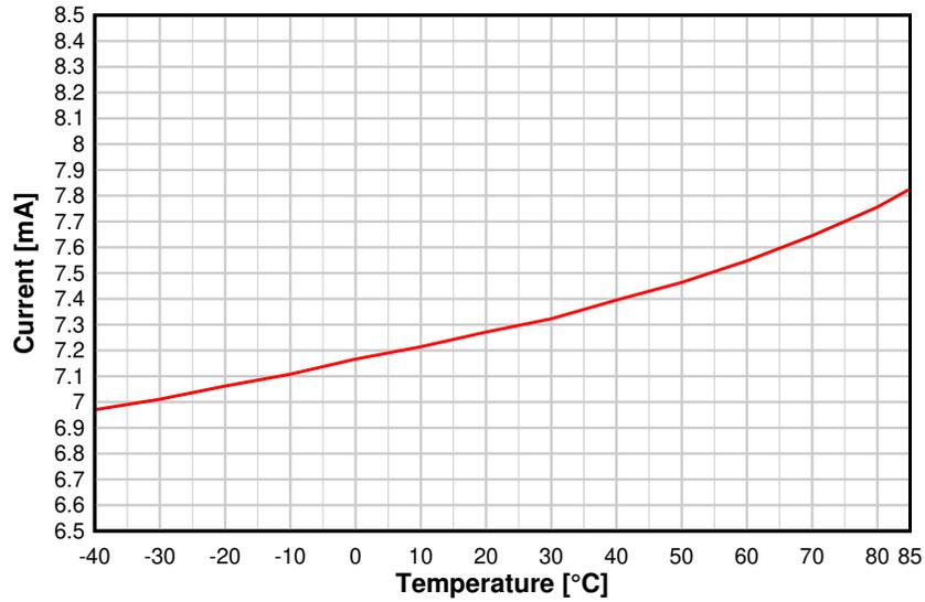
Figure 8-7. RX Current vs. Temperature (BLE 1 Mbps, 2.44 GHz)
