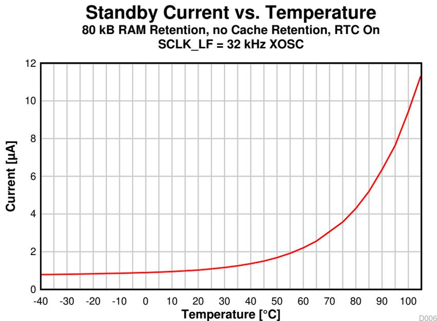
**Figure 8-5. Standby Mode (MCU) Current vs. Temperature**
