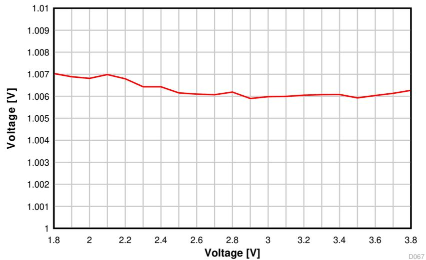
Figure 8-30. ADC Accuracy vs. Supply Voltage (VDD5)
