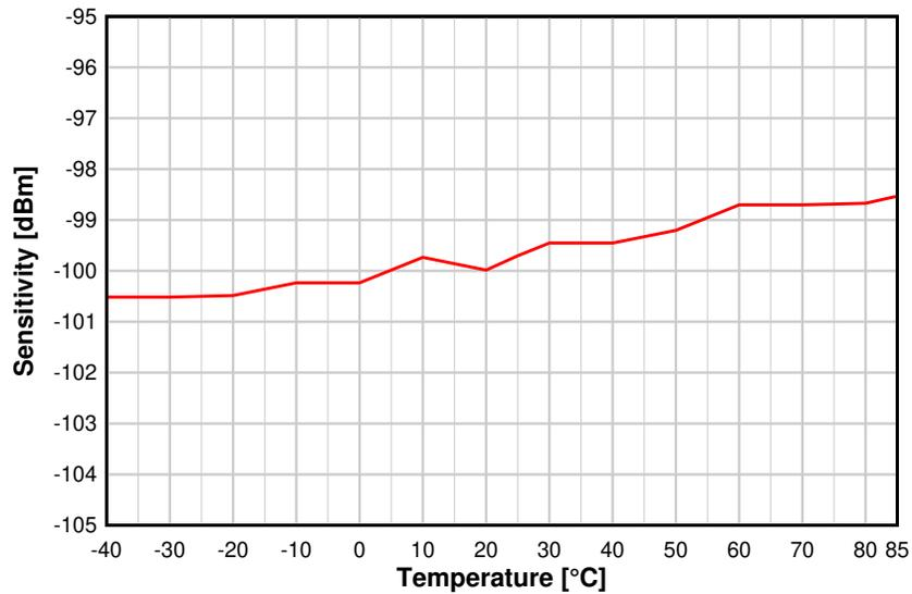
Figure 8-14. Sensitivity vs. Temperature IEEE 802.15.4 (OQPSK DSSS1:8, 250 kbps)
