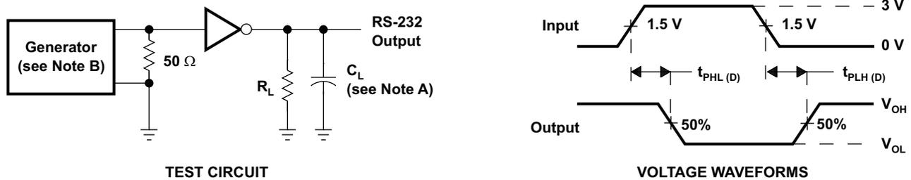
NOTES: A.  $C_L$  includes probe and jig capacitance.
