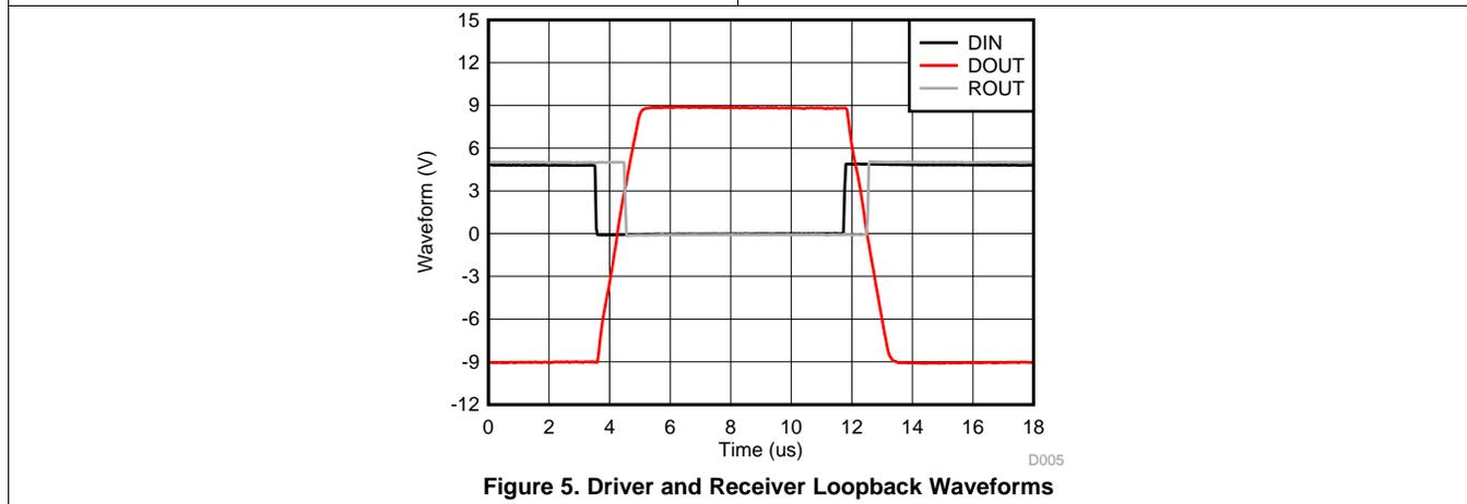
**Figure 5. Driver and Receiver Loopback Waveforms**
