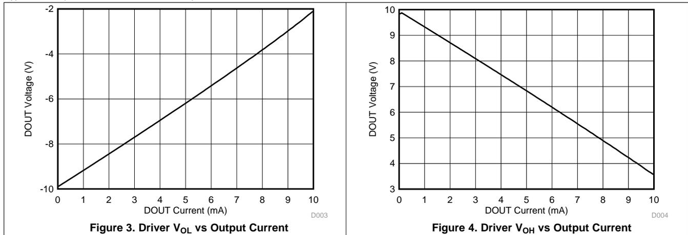
**Figure 3. Driver V<sub>OL</sub> vs Output Current**
