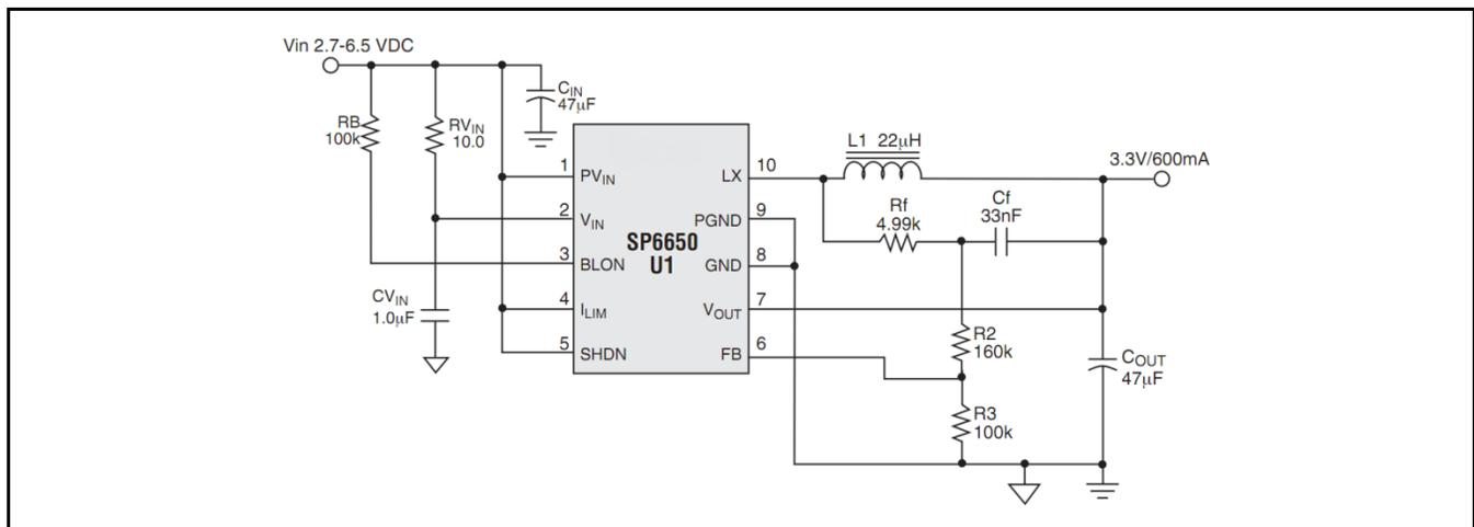
Fig. 19: Additional Application Circuit with Low Output Ripple
