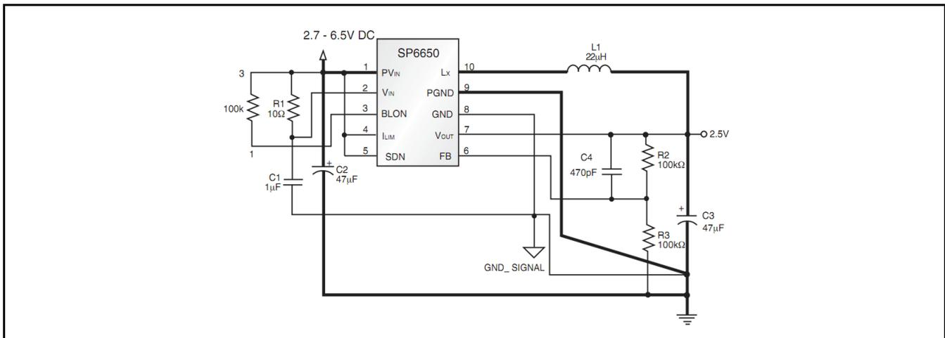
Fig. 24: Application circuit with highlighted power traces.
