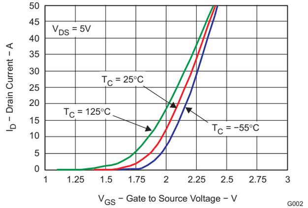
**Figure 3. Transfer Characteristics**
