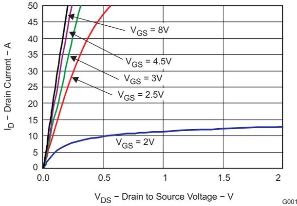
**Figure 2. Saturation Characteristics**
