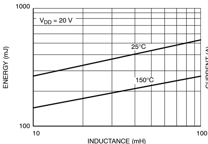
Figure 8. NCV8408 Maximum Switch Off Energy vs Inductance
