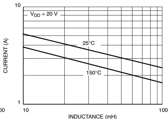
Figure 9. NCV8408 Maximum Switch Off Current vs Inductance
