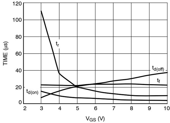
Figure 14. Resistive Switching
