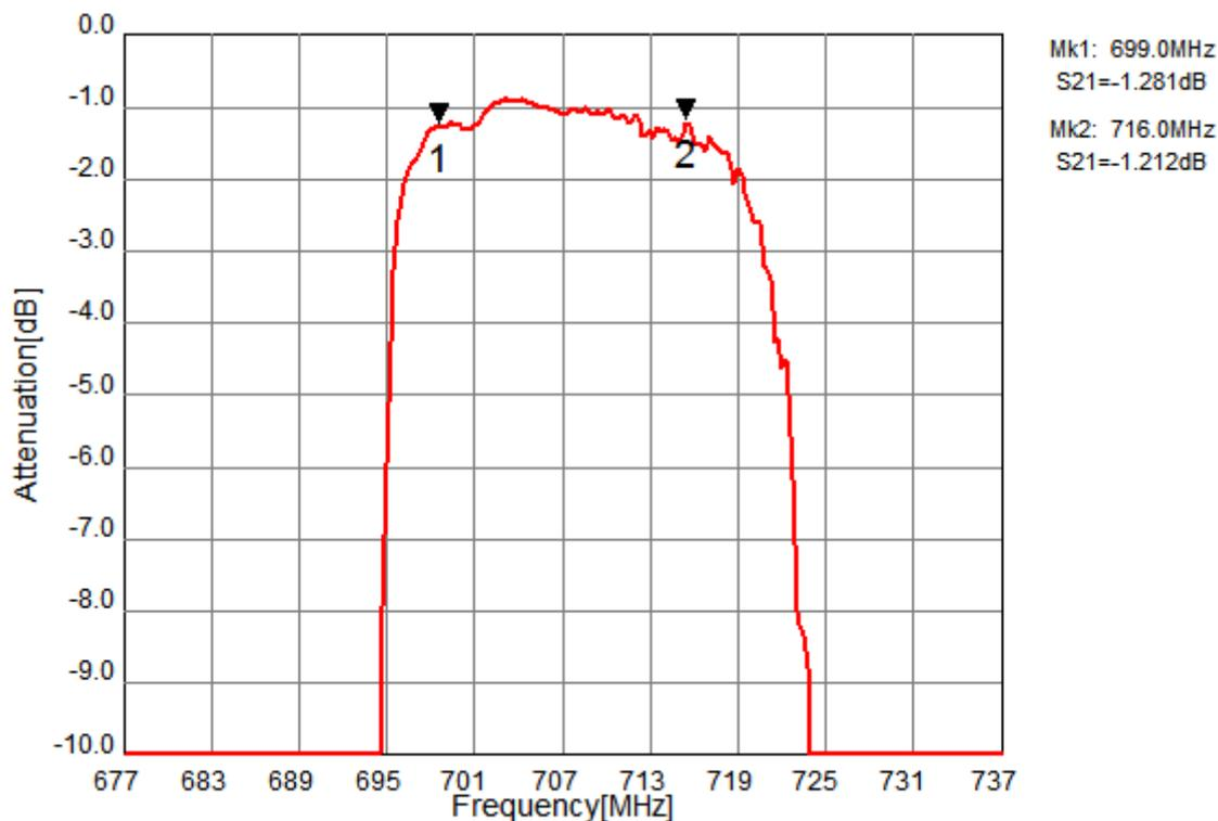
Fig.2 In-band Characteristics
