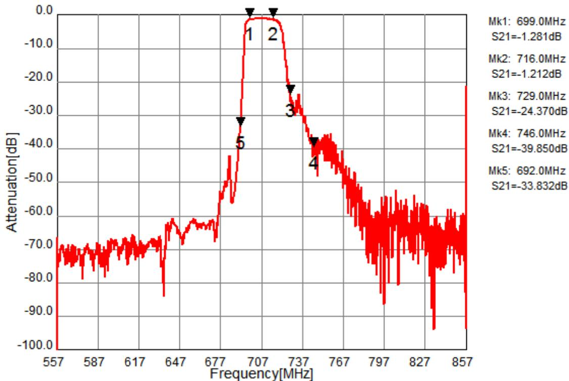
Fig.1 Pass-band Characteristics
