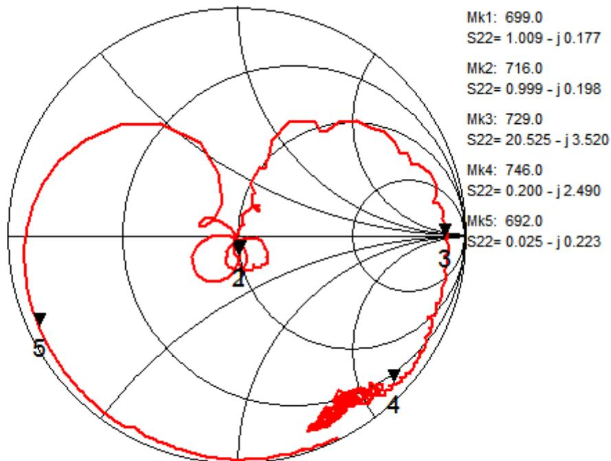
Fig.6 Output Impedance
