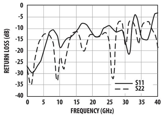
Figure 7. Return Loss (Input and Output).
