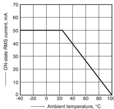
1-(3). ON-state RMS current vs. ambient temperature characteristics
