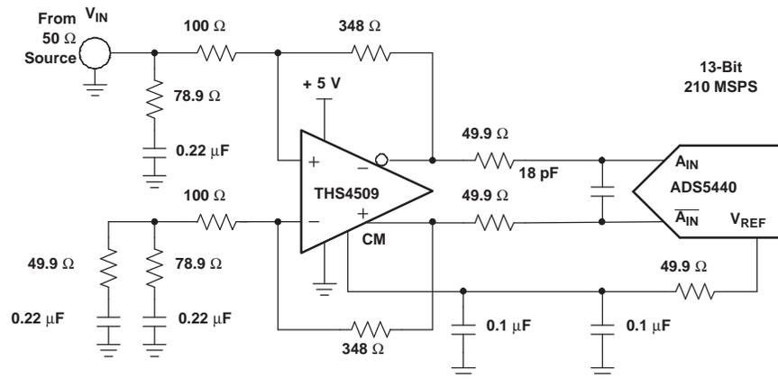
Figure 38. Using the THS4509 With the ADS5440
