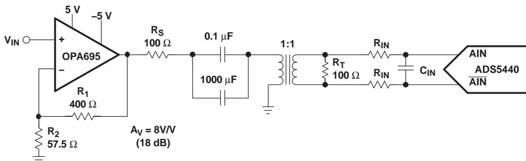
Figure 37. Using the OPA695 With the ADS5440
