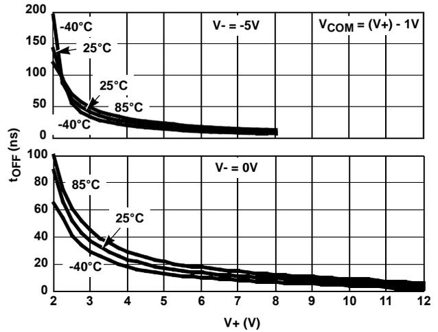
FIGURE 15. ENABLE TURN - OFF TIME vs SUPPLY VOLTAGE
