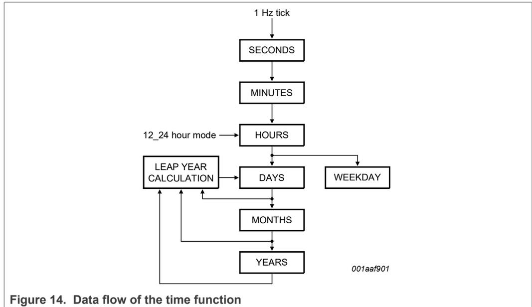
Figure 14. Data flow of the time function
