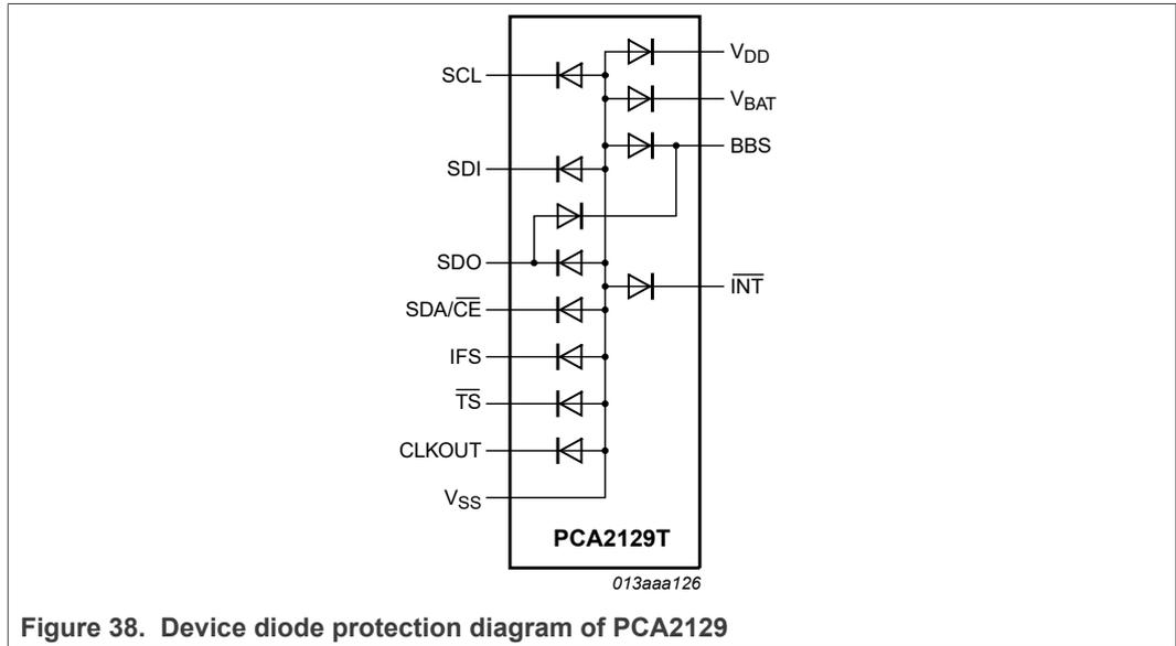
Figure 38. Device diode protection diagram of PCA2129
