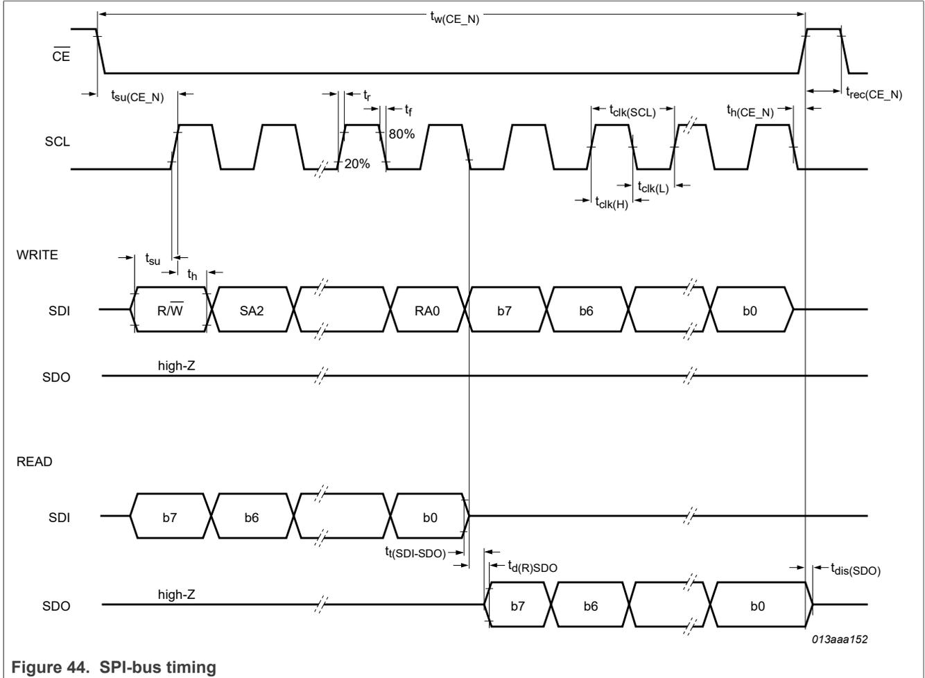
Figure 44. SPI-bus timing
