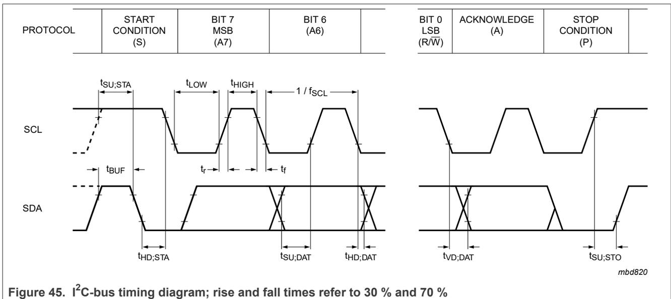
**Figure 45. I<sup>2</sup>C-bus timing diagram; rise and fall times refer to 30 % and 70 %**
