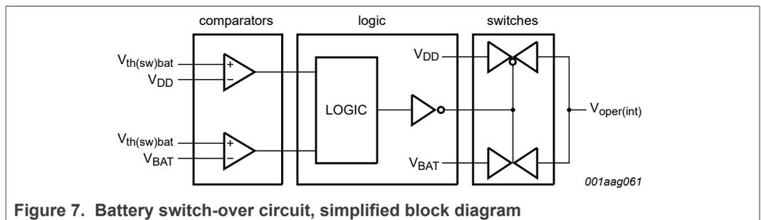
V<sub>oper(int)</sub> is at V<sub>DD</sub> or V<sub>BAT</sub> potential.
