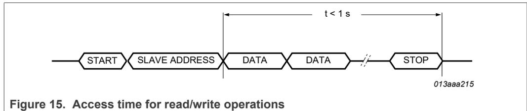
Figure 15. Access time for read/write operations
