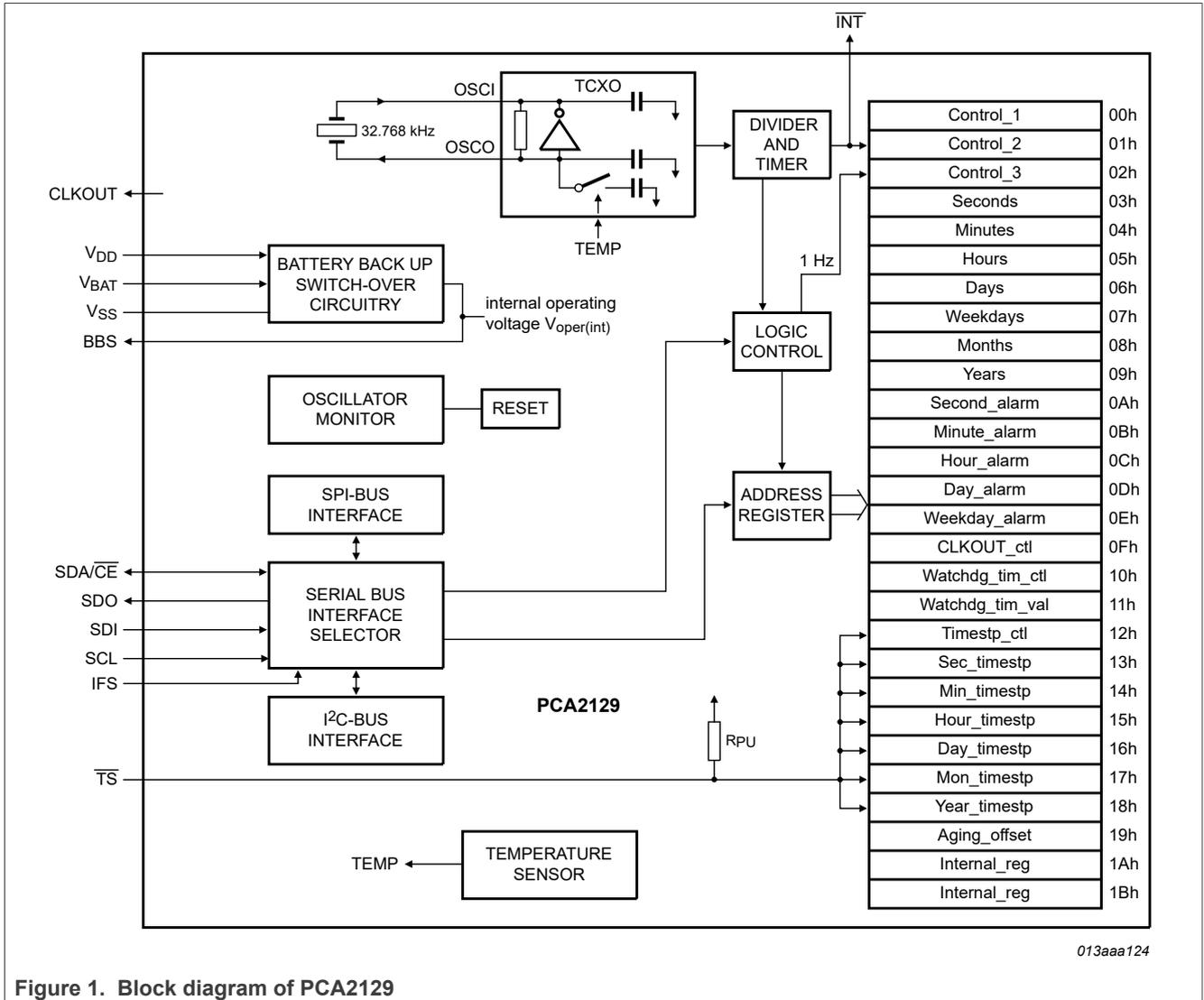
Figure 1. Block diagram of PCA2129
