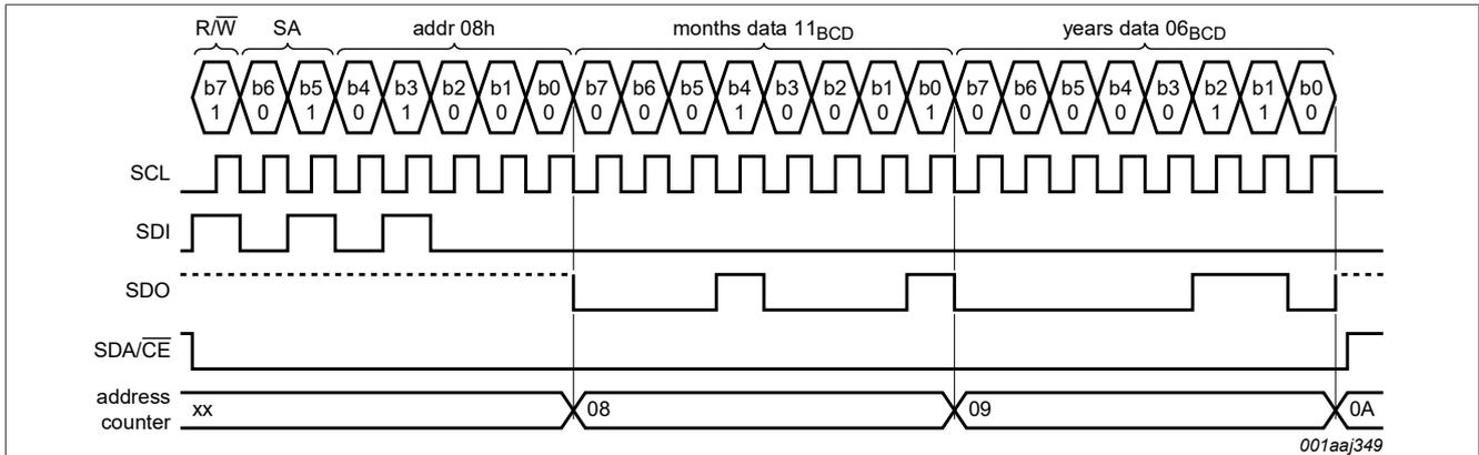
In this example, the registers Months and Years are read. The pins SDI and SDO are not connected together. For this configuration, it is important that pin SDI is never left floating. It must always be driven either HIGH or LOW. If pin SDI is left open, high I<sub>DD</sub> currents may result.
