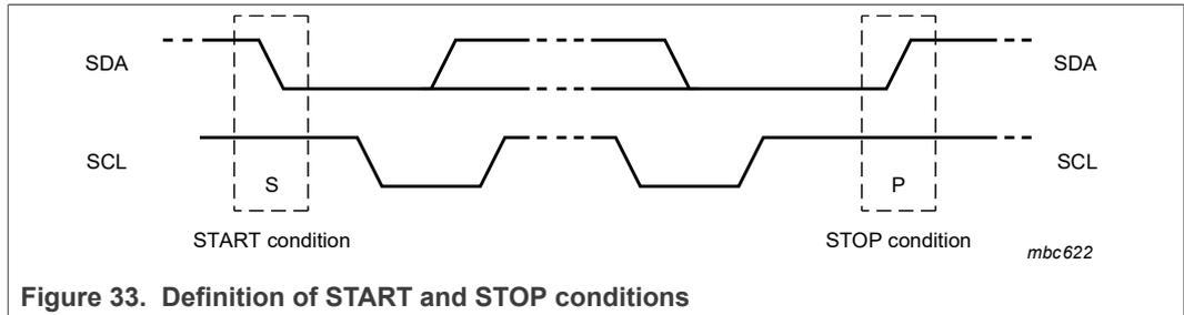
Figure 33. Definition of START and STOP conditions
