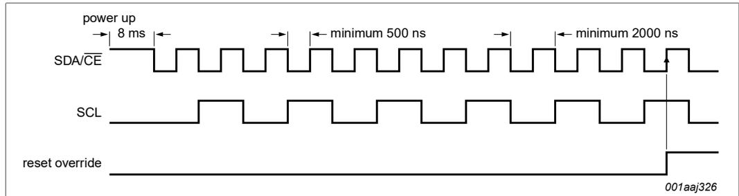
Figure 13. Power-On Reset Override (PORO) sequence, valid for both I<sup>2</sup>C-bus and SPI-bus
