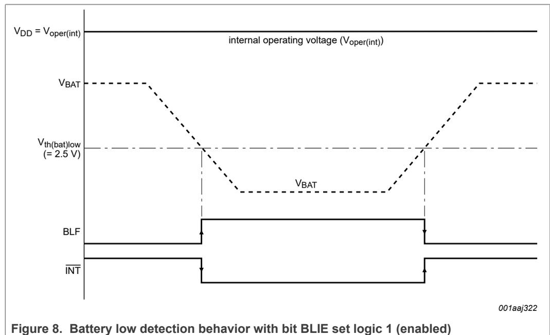
Figure 8. Battery low detection behavior with bit BLIE set logic 1 (enabled)
