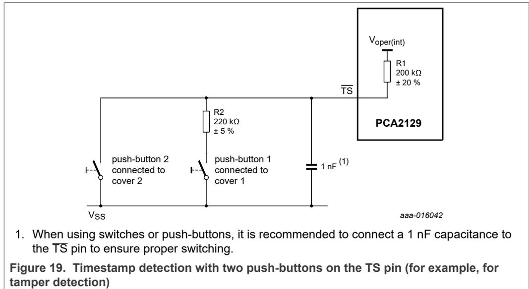
The timestamp function is enabled by default after power-on and it can be switched off by setting the control bit TSOFF (register Timestp\_ctl).
