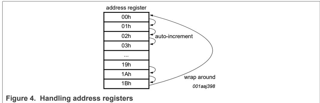
Figure 4. Handling address registers
