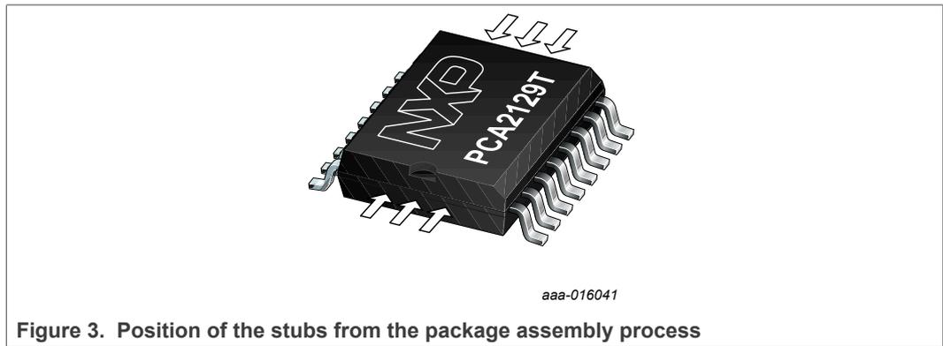
After lead forming and cutting, there remain stubs from the package assembly process. These stubs are present at the edge of the package as illustrated in [Figure 3](#). The stubs are at an electrical potential. To avoid malfunction of the PCA2129, it has to be ensured that they are not shorted with another electrical potential (e.g. by condensation).
