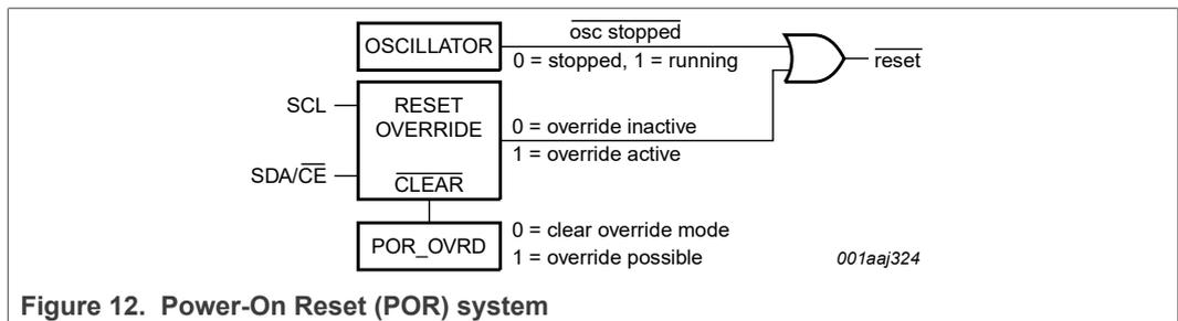
The setting of the PORO mode requires that POR\_OVRD in register Control\_1 is set logic 1 and that the signals at the interface pins SDA/C<sub>E</sub> and SCL are toggled as illustrated in [Figure 13](#). All timings shown are required minimum.
