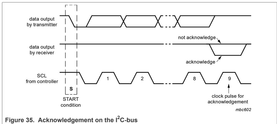
Figure 35. Acknowledgement on the I<sup>2</sup>C-bus
