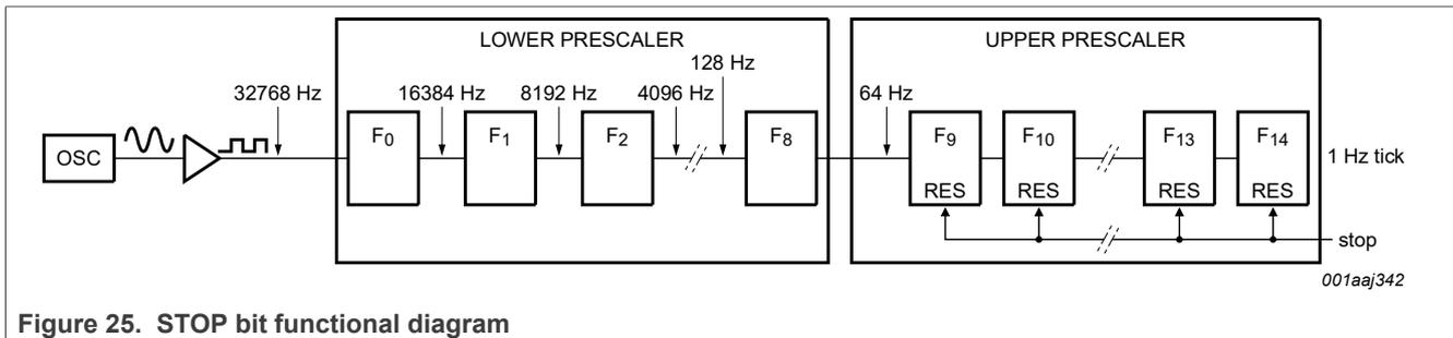
The lower stages of the prescaler, F<sub>0</sub> to F<sub>8</sub>, are not reset and because the I<sup>2</sup>C-bus and the SPI-bus are asynchronous to the crystal oscillator, the accuracy of restarting the time circuits is between 0 and one 64 Hz cycle (0.484 375 s and 0.500 000 s), see [Table 72](#) and [Figure 26](#).
