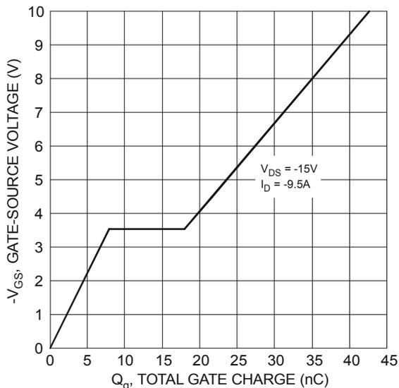
Figure 11 Gate-Charge Characteristics
