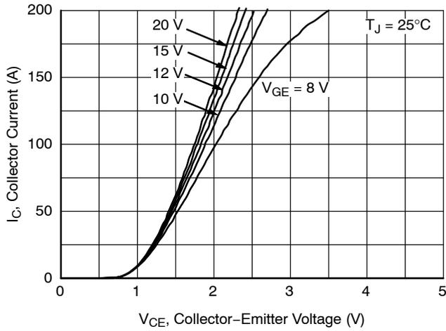
Figure 1. Typical Output Characteristics ( $T_J = 25^\circ\text{C}$ )
