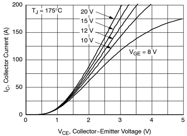
Figure 2. Typical Output Characteristics ( $T_J = 175^\circ\text{C}$ )
