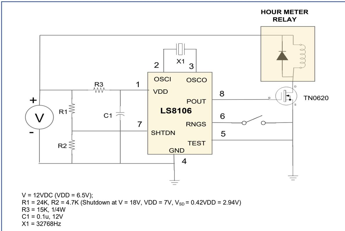
Fig 2. Hour Meter application with output shutdown
