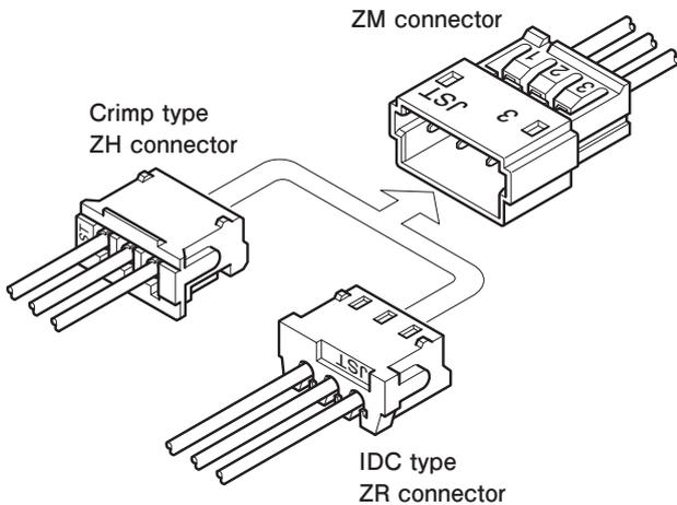
This is a space-saving 1.5 mm pitch wire-to-wire connector that mates with both crimp and IDC type sockets.
