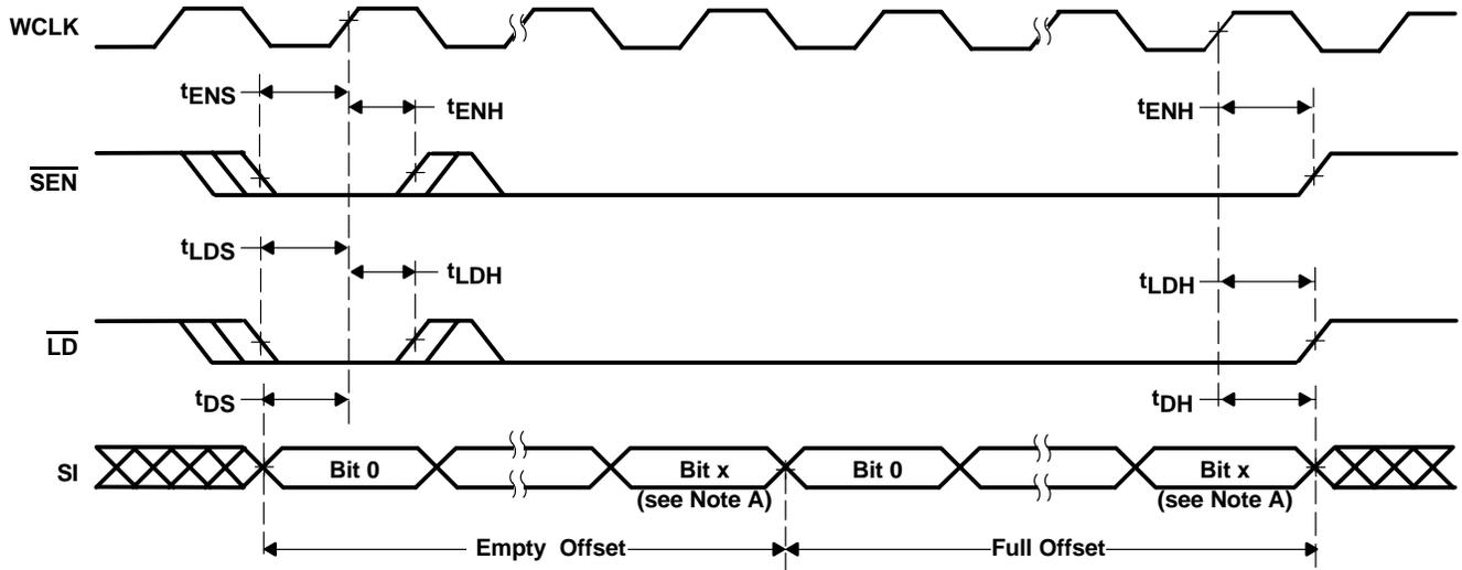
NOTE A: x = 9 for the SN74V3640, x = 10 for the SN74V3650, x = 11 for the SN74V3660, x = 12 for the SN74V3670, x = 13 for the SN74V3680, x = 14 for the SN74V3690.
