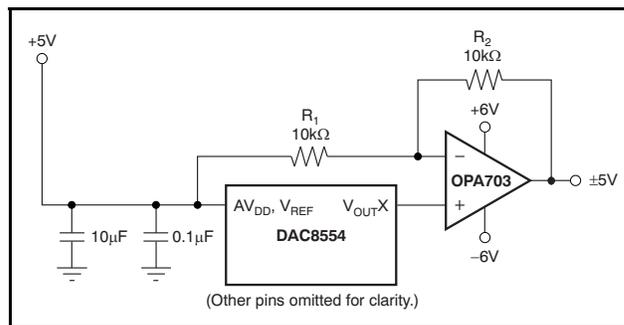
Figure 55. Bipolar Operation With the DAC8554
