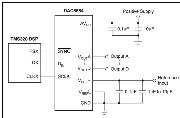
Figure 53. DAC8554 to TMS320 DSP
