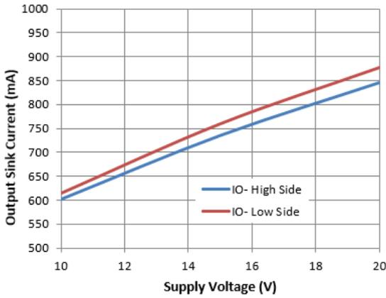
**Figure 17.** Output Sink Current vs. Supply Voltage
