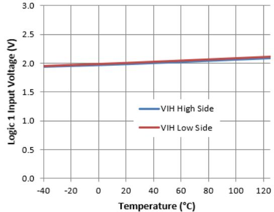
**Figure 20.** Logic 1 Input Voltage vs. Temperature
