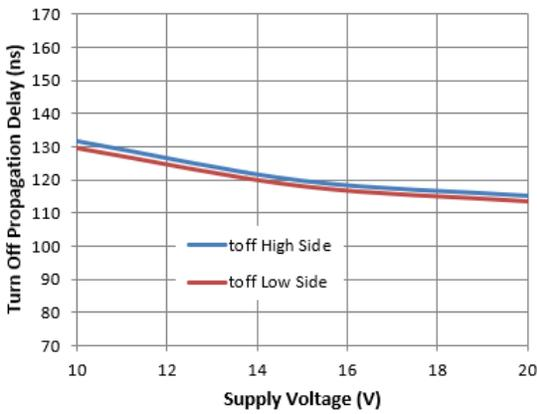
**Figure 5.** Turn-off Propagation Delay vs. Supply Voltage
