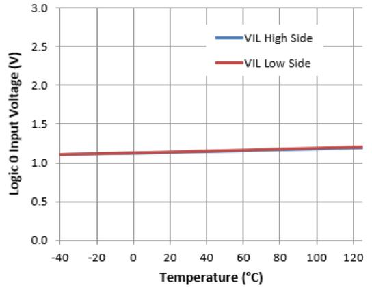
**Figure 22.** Logic 0 Input Voltage vs. Temperature
