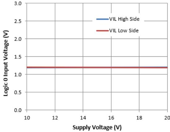
**Figure 21.** Logic 0 Input Voltage vs. Supply Voltage
