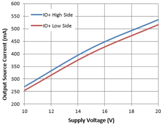
**Figure 15.** Output Source Current vs. Supply Voltage
