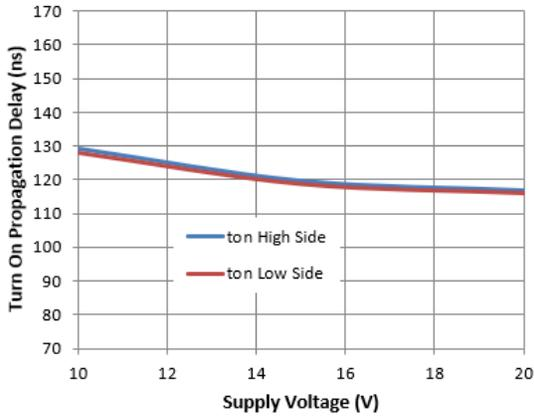
**Figure 3.** Turn-on Propagation Delay vs. Supply Voltage
