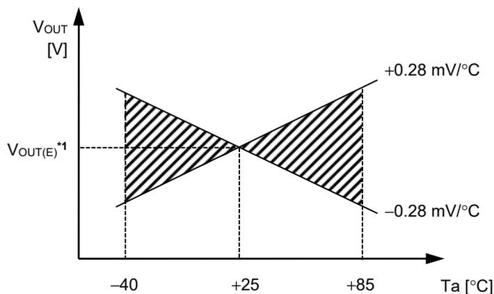
\*1.  $V_{OUT(E)}$  is the value of the output voltage measured at  $T_a = +25^{\circ}\text{C}$ .
