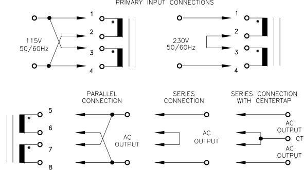
\*not UL - recognized for series connect.
